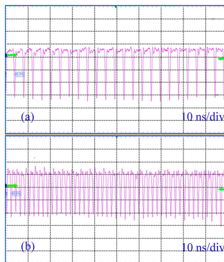
FIG. 6. Oscilloscope traces of the dark pulse emission of the laser. I = 120 mA, L_{\text{ext}} = 61 cm. (a) single dark pulse in cavity with a repetition rate of 244 MHz. (b) Two dark pulses in cavity with a repetition rate of 488 MHz.
