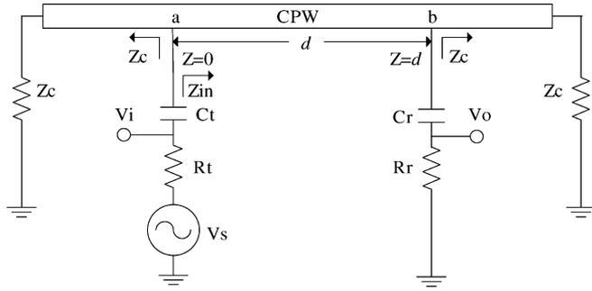
Fig. 2. Channel model:  $C_t$  is the transmitter's coupling capacitor,  $C_r$  is the receiver's coupling capacitor,  $R_t$  is the transmitter's output resistance,  $R_r$  is the receiver's input resistance,  $V_s$  is the source signal voltage,  $d$  is the distance between the transmitter and receiver,  $Z_{in}$  is the impedance looked into the CPW,  $V_i$  is the channel's input voltage, and  $V_o$  is the channel's output voltage.
