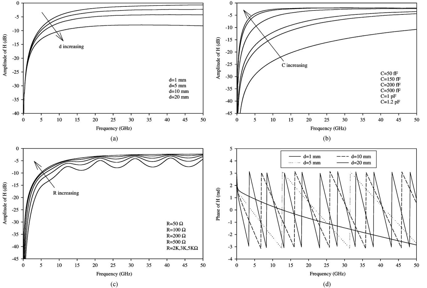
Fig. 3. Amplitude and phase of  $H$  versus frequency. (a) Effect of distance:  $C = 500$  fF,  $R = 5$  k $\Omega$ . (b) Effect of coupler capacitance:  $d = 5$  mm,  $R = 5$  k $\Omega$ . (c) Effect of resistance:  $d = 5$  mm,  $C = 500$  fF. (d) Effect of distance:  $C = 500$  fF,  $R = 5$  k $\Omega$ .
