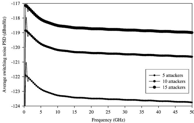
Fig. 9. Average switching noise PSD versus frequency.
