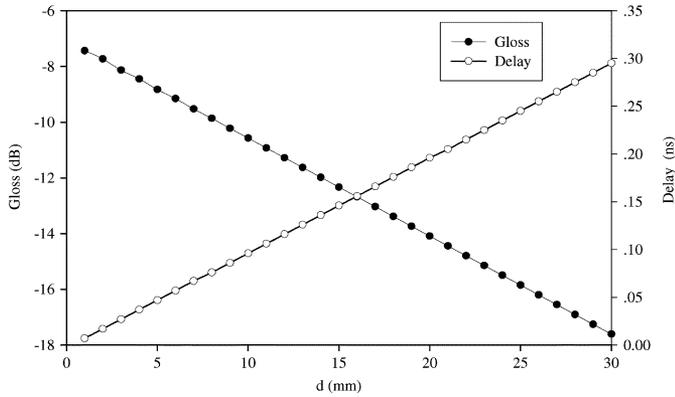
Fig. 6. Received signal's delay and energy loss versus distance.
