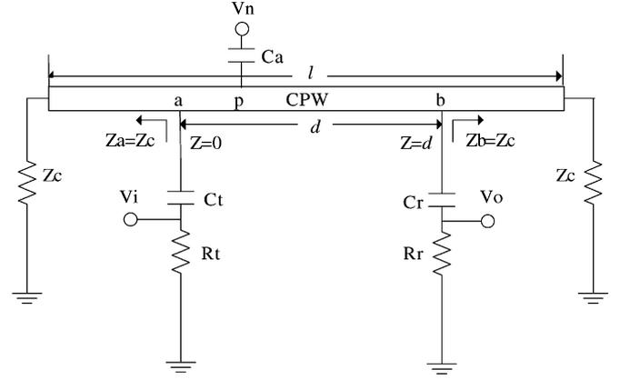
Fig. 7. Switching noise attack model.
