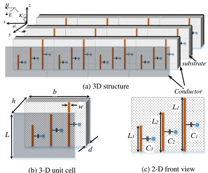
Fig. 1. Structure of the proposed multi-band FSS.
