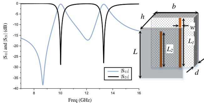
Fig. 2. Unit cell of a dual-band FSS and simulated transmission and reflection coefficients ( $b=6\text{mm}$ ,  $h=3.524\text{mm}$ ,  $L=9.5\text{mm}$ ,  $d=1.524$ ,  $w=0.3\text{mm}$ ,  $L_1=9.5\text{mm}$ ,  $L_2=6.5\text{mm}$ ,  $\epsilon_r=3.55$ ).
