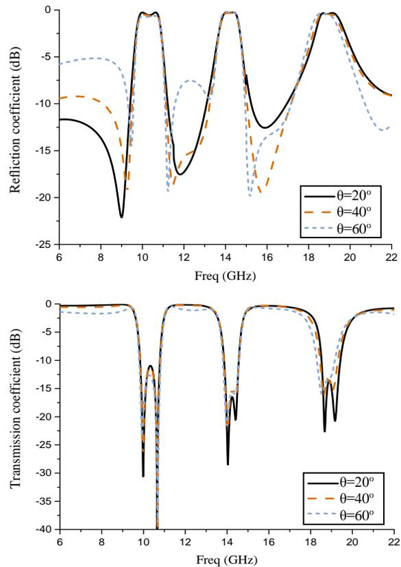
Fig. 4. Simulated transmission and reflection coefficients of a tri-band FSS with different incident angles.
