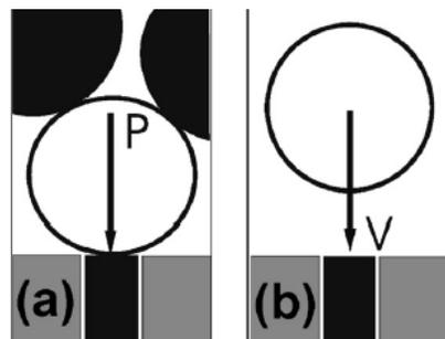
Figure 13: Impact modes of media: a) longer duration non-impact contacts and b) short duration direct impacts [35]
