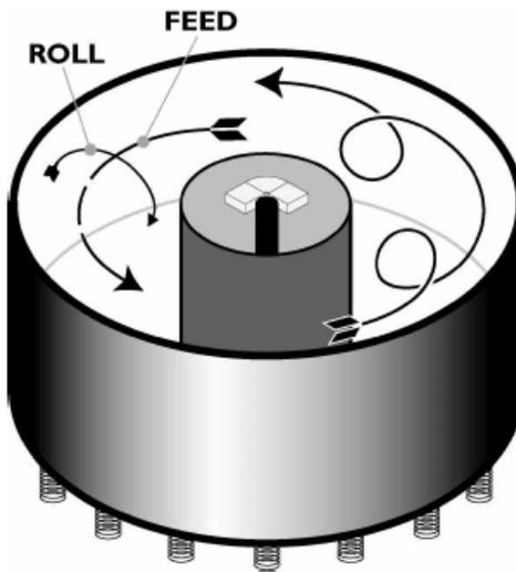
Figure 6: Roll and feed motions in a vibratory bowl [13]
