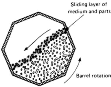
Vibrating barrels produce better surface finish
