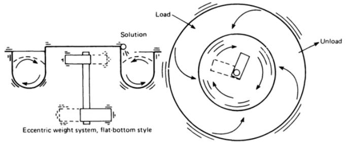
High speed rotating disc produces faster finishing action
