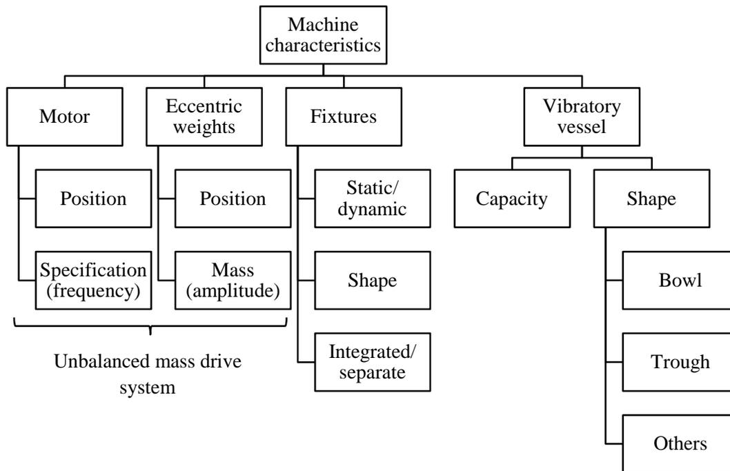
Figure 5: Vibratory finishing machine characteristics
