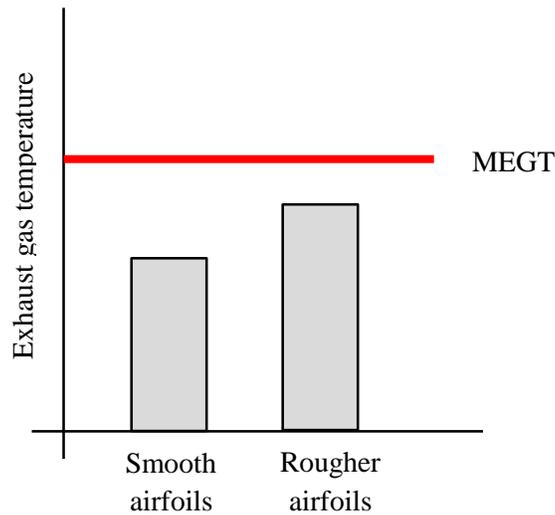
Figure 3: The effect of surface finish on aircraft engine exhaust gas temperatures
