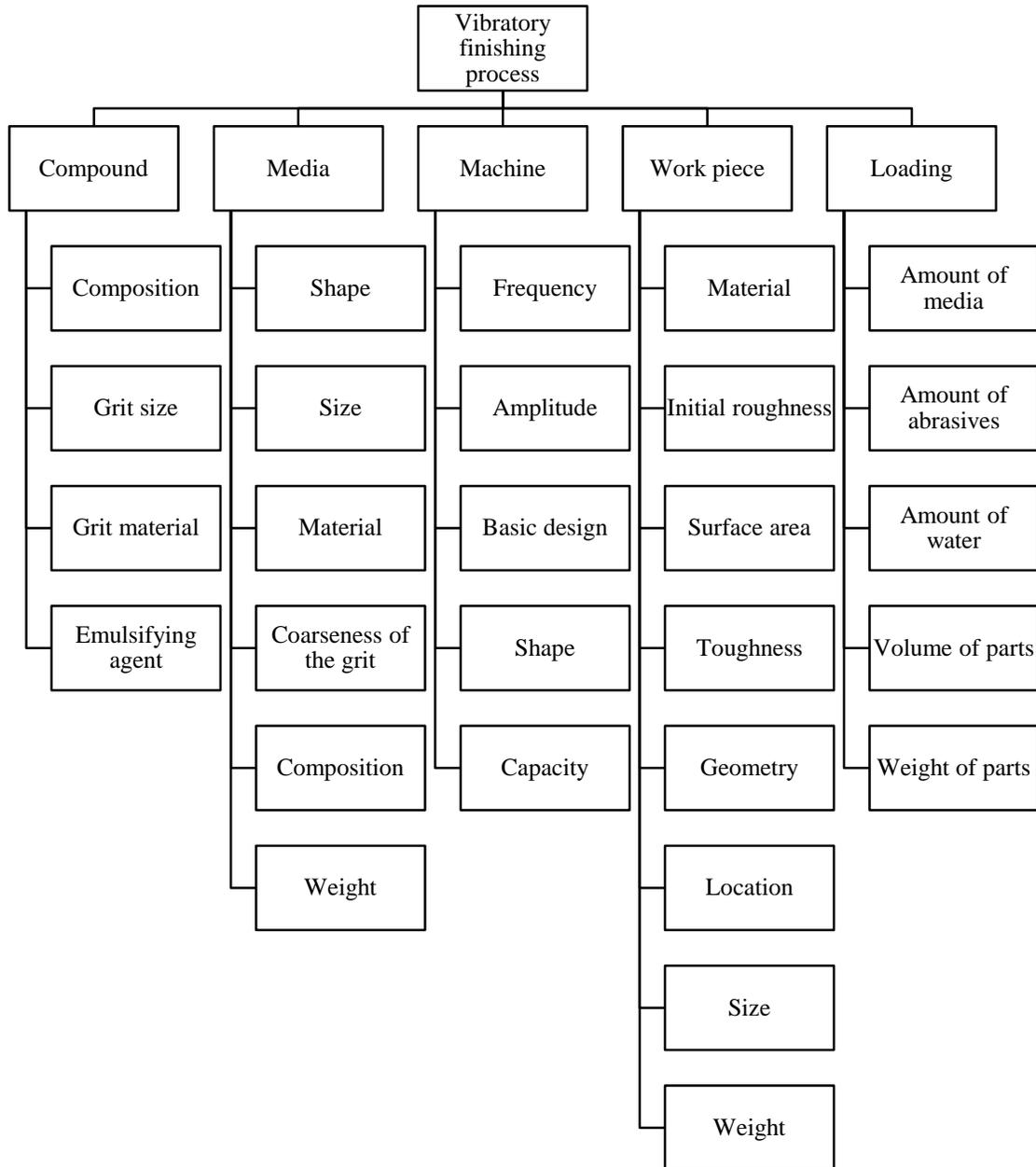
Figure 4: Vibratory finishing KPVs [3]
