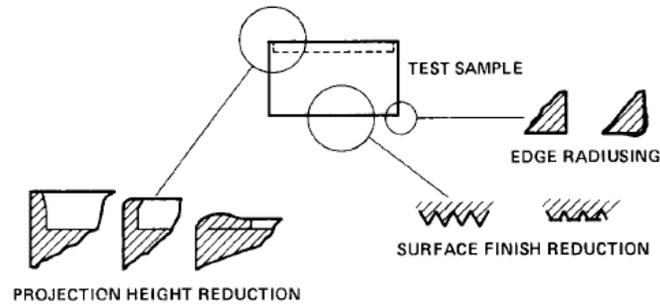
Figure 12: Projection height reduction, surface finish reduction and edge radiusing in a workpiece [31]
