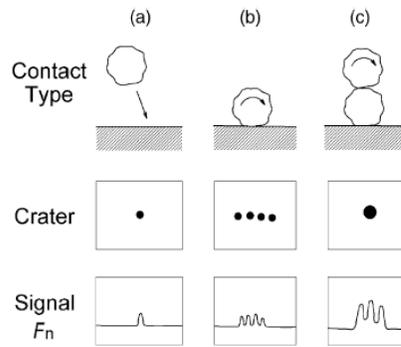
Figure 11: Contact modes of media in vibratory finishing: a) free impact, b) rolling of individual media and c) adjacent media rolling over a stationary piece of media [1]
