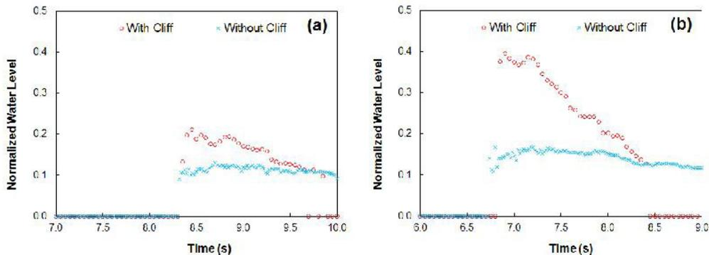
Fig. 6. Comparison of the water levels during the contact period at the toe of the cliff for  $H_0 =$  (a) 0.025 m and (b) 0.055 m with and without the presence of the steep cliff. The results are from simulations with particle size of 0.005 m. The normalized water level are normalized by the mean water depth  $d$ .
