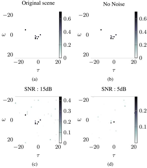
**Fig. 1.** CS radar simulations with  $K = 8$  targets on a  $47 \times 47$  time-frequency plane at various noise levels. (a) Original scene; CS reconstructions with (b) No noise, (c) SNR=15 dB, and (d) SNR=5 dB.
