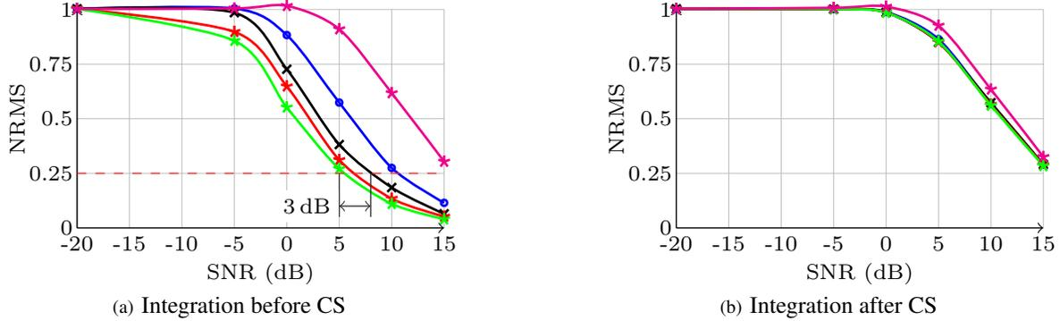
**Fig. 3.** Reconstruction error performance for integration (a) before, and (b) after CS reconstruction for the different coherent integration durations,  $N=1$  (magenta),  $N=5$  (blue),  $N=10$  (black),  $N=15$  (red), and  $N=20$  (green). Sparsity level is  $K = 8$  with cell size of  $47 \times 47$ . NRMS stands for normalized root-mean-square between original and reconstructed target scene.
