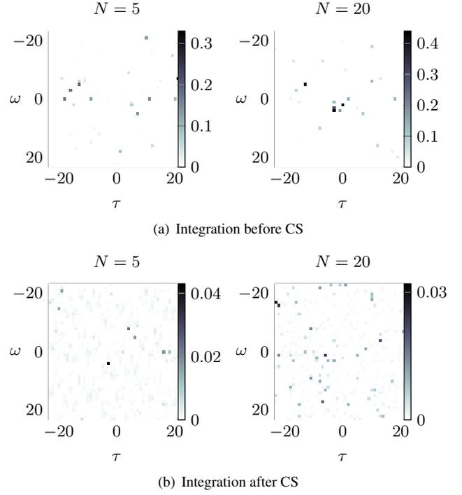
**Fig. 2.** CS radar simulations along with coherent integration of the original scene shown in Fig. 1(a). The noise of single radar return is SNR = 0 dB. (a) Integration is performed before CS, and (b) Integration is performed after CS.
