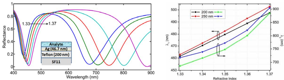
Fig. 4. (a) SPR curves for varying analyte refractive indices at optimum Ag/Teflon structure, (b) Response curves for nearly optimum SF11/Cytop/Ag structure at 53.5° angle of incidence.
