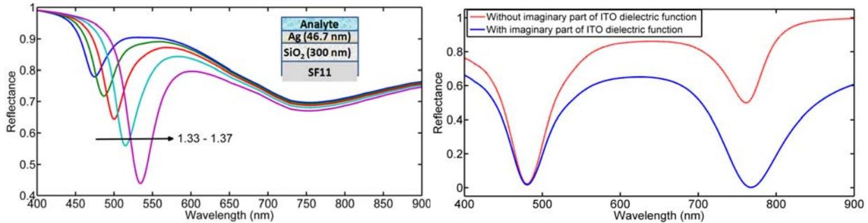
Fig. 3. (a) SPR curves for varying refractive indices of the analyte at the optimum self-referencing Ag/SiO<sub>2</sub> structure at 57° angle of incidence, (b) Effect of the imaginary part of dielectric function of ITO on the SPR response.
