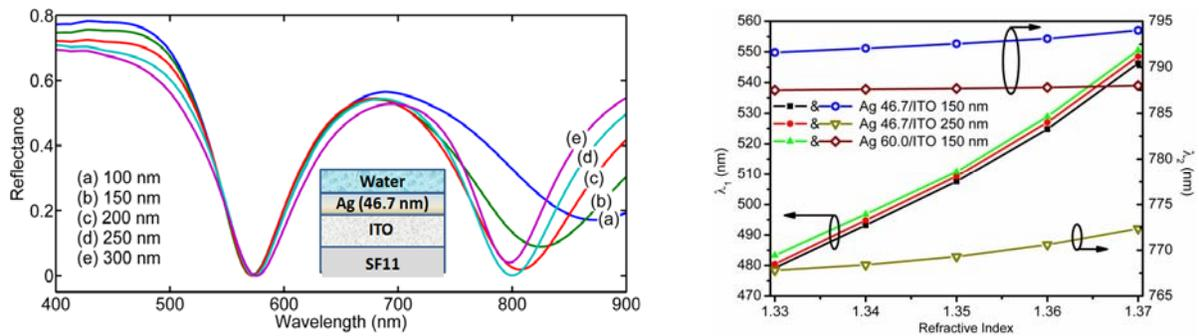
Fig. 2. (a) SPR spectra for varying thicknesses of ITO at 53.5° angle of incidence and 46.7 nm thickness of Ag film. The spectra are used for the optimization of ITO thickness. (b) Response curves for nearly optimum structures: Optimization of Ag thickness for self-referencing.
