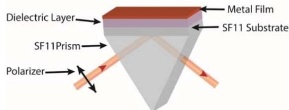
Fig. 1. Schematic of dual mode SPR geometry in a Kretschmann configuration
