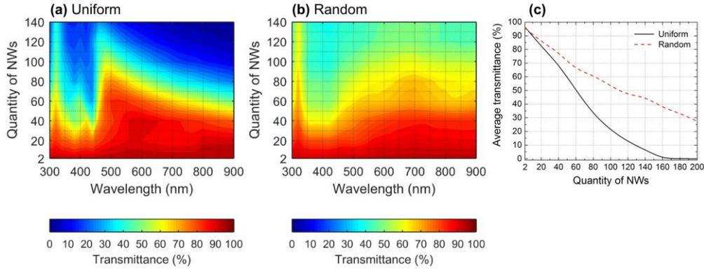
Fig. 2. Dependence of the transmittance of Ag NW layers on the quantity of NWs per area of  $8 \times 8 \mu\text{m}^2$  with the uniform (a) and random (b) arrangement for the wavelength range from 300 to 900 nm. (c) Dependence of the average transmittance in visible spectrum on the quantity of NWs per area of  $8 \times 8 \mu\text{m}^2$  for uniform and random arranged Ag NW layers.
