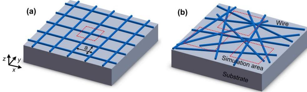
Fig. 1. Geometrical models of uniformly (a) and randomly (b) arranged NW layers on the glass substrate. Red rectangles are the unit simulation areas, which are equal to  $a^2$  and  $8 \times 8 \mu\text{m}^2$  for the NWs with uniform and random arrangement, respectively.
