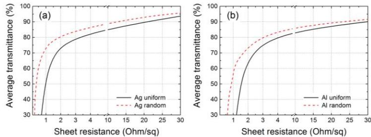
Fig. 5. Sheet resistance versus average transmittance in visible wavelength spectrum for *Al* (left) and *Ag* (right) uniformly and randomly arranged NWs layers.
