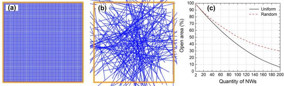
Fig. 3. The distribution of the uniform (a) and random (b) NWs for the quantity of 140 per  $8 \times 8 \mu\text{m}^2$ . (c) Dependence of the open area on the quantity of NWs per  $8 \times 8 \mu\text{m}^2$  for the uniform and random NW layers.
