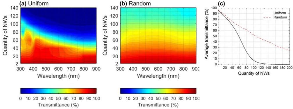
Fig. 4. Dependence of the transmittance of *Al* NW layers on the quantity of NWs per area of  $8 \times 8 \mu\text{m}^2$  with the uniform (a) and random (b) arrangement for the wavelength range from 300 to 900 nm. (c) Dependence of the average transmittance in visible spectrum on the quantity of NWs per area of  $8 \times 8 \mu\text{m}^2$  for uniform and random arranged *Al* NW layers.
