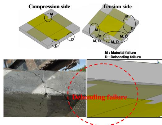
Figure 4: Analytical prediction of the local debonding failure
