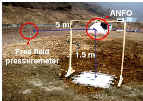
Figure 1: Blast test setup
