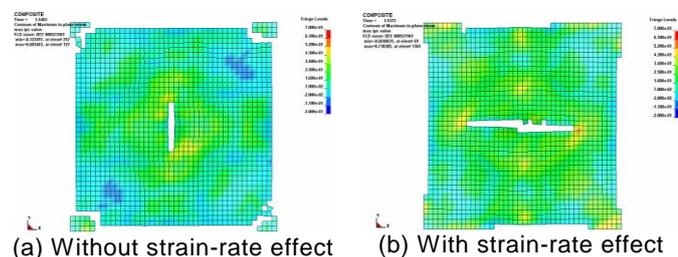
Figure 2: Comparison of max. in-plane stress distribution according to strain rate dependency
