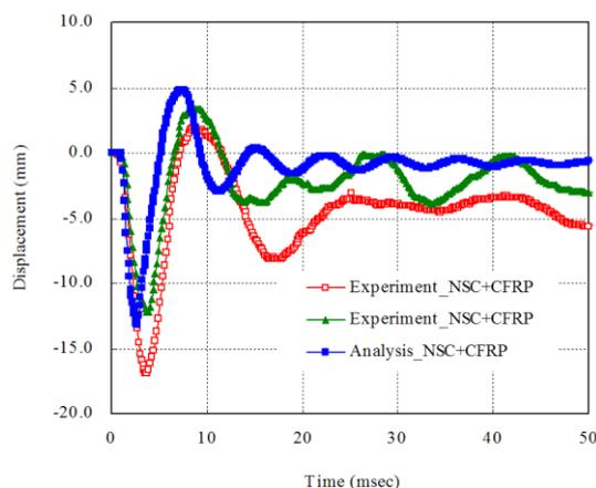
Figure 3: CFRP retrofitted displacement behavior
