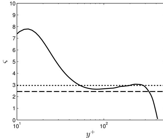
Figure 7: The indicator function,  $\zeta = y^+ du^+ / dy^+$ . (—) DNS data from Touber and Leschziner (2012); (···) Line indicating the value  $1/\kappa r$ ; (- -) Line indicating the value  $1/\kappa$ .
