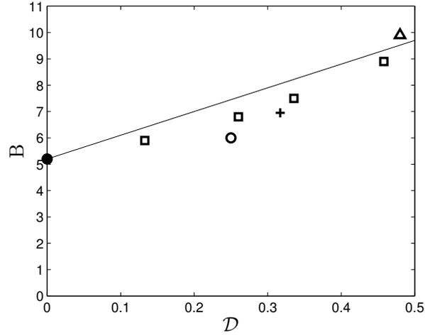
Figure 6: The additive constant  $B$  as a function of DR.  $\bullet$  Reference case at  $Re_\Theta = 1190$ ;  $\square$  DR cases at  $Re_\Theta = 1190$ .  $\circ$  at  $Re_\Theta = 1400$ ;  $+$  at  $Re_\Theta = 1374$ ;  $\Delta$  at  $Re_\Theta = 464$ . The solid line is Eq. (16) for  $Re_\Theta = 505$ .
