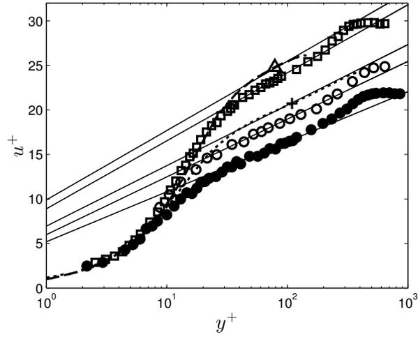
Figure 5: Velocity profiles scaled with actual friction velocity  $u_\tau$ . Experimental data taken from Choi and Clayton (2001):  $\bullet$  Reference case;  $\square$  DR case with  $\mathcal{D} = 0.46$ .  $\circ$  Experimental data taken from Ricco and Wu (2004).  $\dots$  (+)DNS data taken from Touber and Leschziner (2012).  $--$  ( $\Delta$ )DNS data taken from Quadrio et al. (2009). Thin solid lines according to Eq. (9).
