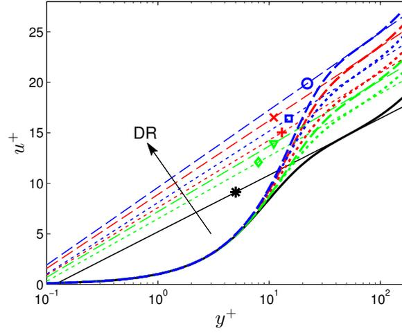
Figure 1: The velocity profiles scaled with actual friction velocity  $u_\tau$ . Thick lines from DNS data; Thin lines (with symbols as in Table 1) according to Eq. (9). (—) Reference case; (---) Spatial forcing; (···) Temporal forcing. Color online: wall forcing amplitude  $W_m^+ = 6$  (green);  $W_m^+ = 12$  (red);  $W_m^+ = 17$  (blue).
