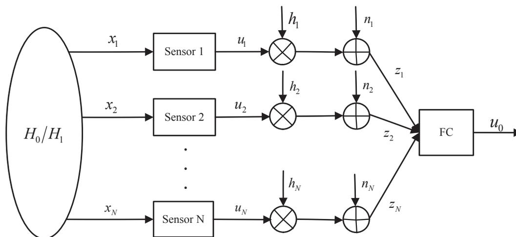
**Figure 1.** A block diagram of the parallel fusion model in the presence of fading and noisy channels between sensors and the fusion center (FC).
