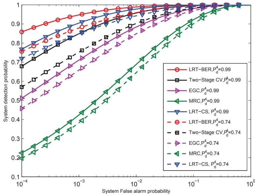
**Figure 8.** ROC curves of LRT-BER, MRC, EGC and LRT-CS statistics with different local detection probabilities and different received SNRs by using the CLT approximation. The local false alarm probability is  $P_{fa} = 0.1$ . BPSK modulation and the Rayleigh fading assumption are considered.
