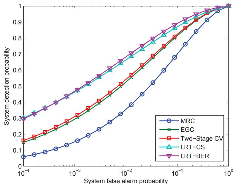
**Figure 6.** Comparison of ROC curves for LRT-BER, maximum ratio combiner (MRC), equal gain combiner (EGC) and LRT-channel statistics (CS) with six sensors,  $\bar{\gamma}_b = 5$  dB,  $P_{fa} = 0.1$ ,  $P_d = 0.6$ . BPSK modulation and Rayleigh fading assumption are considered.
