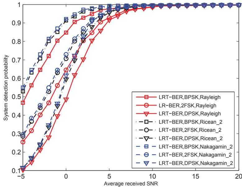
**Figure 4.** Detection probability of the LRT-BER fusion rule as a function of different received SNRs for BPSK, 2FSK and DPSK modulations with  $N = 20$ . Rayleigh fading, Ricean fading with factor  $K = 2$  and Nakagami- $m$  fading with  $m = 2$  are considered.  $P_{fa} = 0.1$ ,  $P_d = 0.6$ , and  $P_{FA} = 0.01$ .
