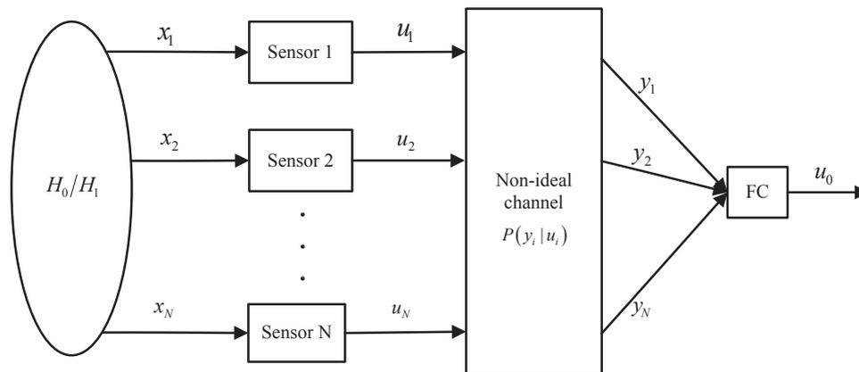
**Figure 2.** A block diagram of parallel fusion model in the presence of the non-ideal channel characterized by  $P(y_i|u_i)$ .
