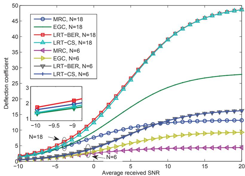
**Figure 7.** Deflection coefficient of MRC, EGC, LRT-CS, two-stage CV and LRT-BER statistics with six and eighteen sensors, respectively,  $P_{fa} = 0.1$ ,  $P_d = 0.6$ . BPSK modulation and the Rayleigh fading assumption are considered.
