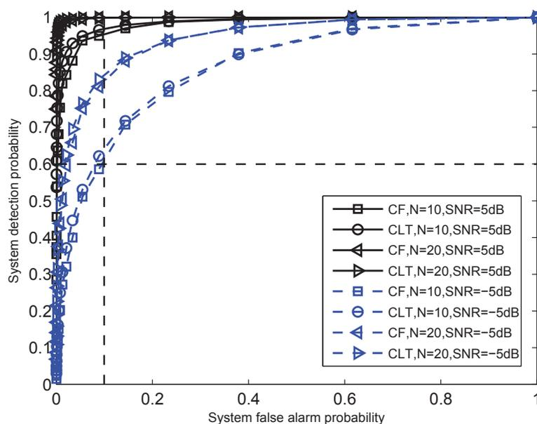
**Figure 3.** ROC curves for the likelihood ratio test (LRT)-bit error (BER) fusion rule based on central limit theorem (CLT) and closed-form (CF) performance evaluation with  $N = 10$  and  $N = 20$ . Average received SNRs are assumed to be SNR =  $-5$  dB and SNR =  $5$  dB. Each local detection index is assumed to be equal to each other ( $P_{fa} = 0.1$ ,  $P_d = 0.6$ ). BPSK modulation is used, and the Rayleigh fading envelope is assumed.
