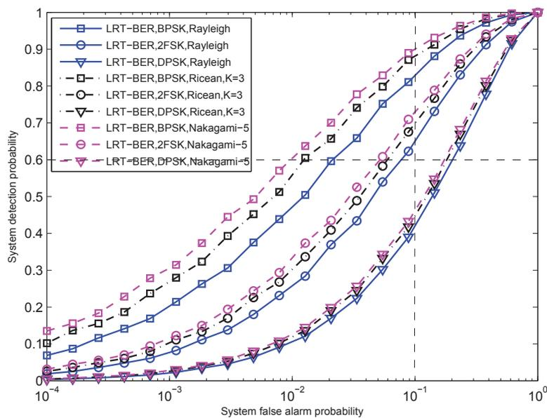
**Figure 5.** ROC curves for the LRT-BER fusion rule based on CF closed-form performance evaluation with  $N = 20$ . The average received SNR is  $\bar{\gamma}_b = -5$  dB. Each local detection index is assumed to be equal to each other ( $P_{fa} = 0.1$ ,  $P_d = 0.6$ ). The system alarm probability is  $P_{FA} = 0.01$ .
