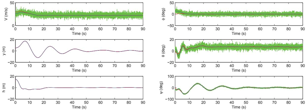
**Figure 4.** Time responses of the velocity ( $V$ ), lateral displacement ( $y$ ), altitude ( $h$ ), roll ( $\phi$ ), pitch ( $\theta$ ) and yaw ( $\psi$ ) angles. Blue, green and red denote actual, estimated and filtered values, respectively.
