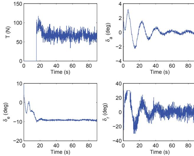
**Figure 5.** Time responses of the thrust ( $T$ ), aileron ( $\delta_a$ ), elevator ( $\delta_e$ ) and rudder ( $\delta_r$ ) deflections.
