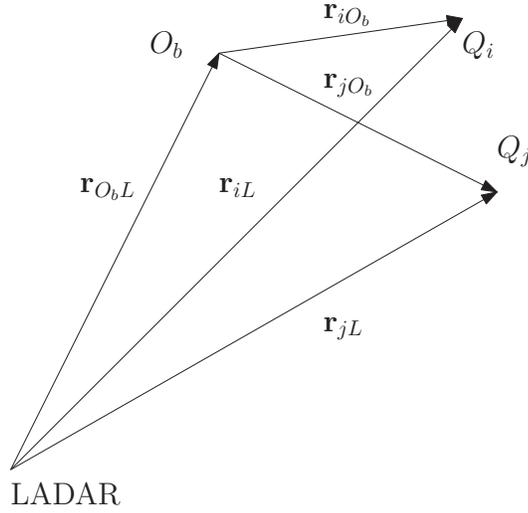
**Figure 1.** Relations between points on the aircraft and their LADAR observations.
