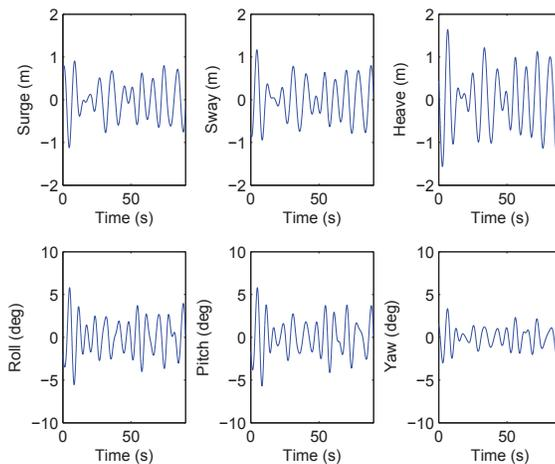
**Figure 2.** Surge, sway, heave, roll, pitch and yaw motions for a barge at 0 kts and heading angle of 135 deg (sea state described by Modified Pierson-Moskowitz spectrum with  $h_{1/3} = 4$  m and  $T = 7$  s).
