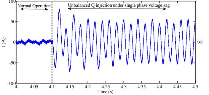
Fig. 10. Performance of the proposed controller under single phase fault: (a) PCC voltage and phase current and (b) Injected active/reactive power, (c) Neutral wire current
