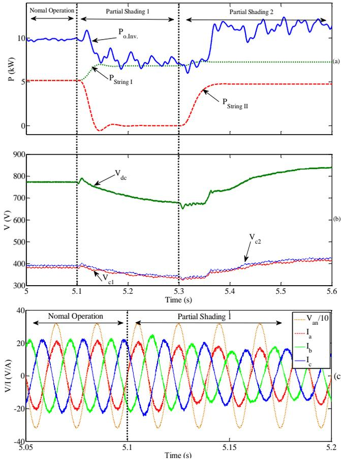
Fig. 7. Dynamic performance of the PV grid connected inverter under various temperature and irradiation conditions: (a) PV string power and inverter output power, (b) DC-link and capacitor voltages and (c) Grid currents and phase voltage.
