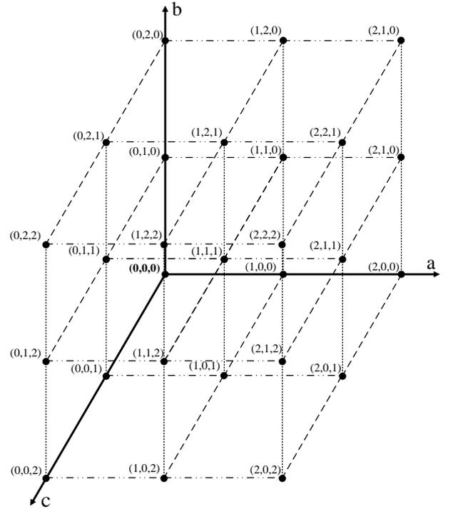
Fig. 3. 3-D space vector representation of the NPC inverter in abc coordinate
