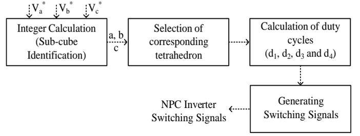
Fig. 5. Flowchart of 3-D SVM for NPC inverter
