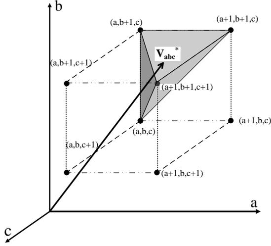
Fig. 4. Tetrahedron into the cube with corresponding state vectors of 3-D SVM
