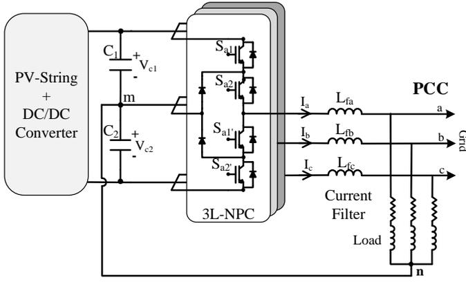
Fig. 1. Proposed Four-Wire Multi-string PV power plant
