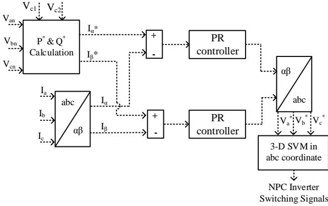
Fig. 2. Proposed VOC-PR Controller with 3-D SVM in abc coordinate
