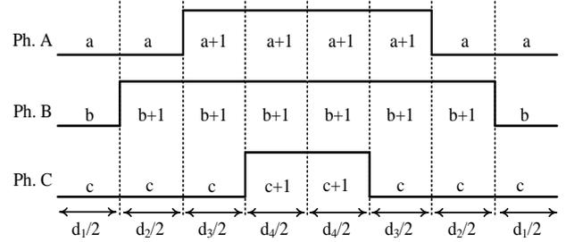
Fig. 6. Switching states of 3-D SVM for NPC inverter
