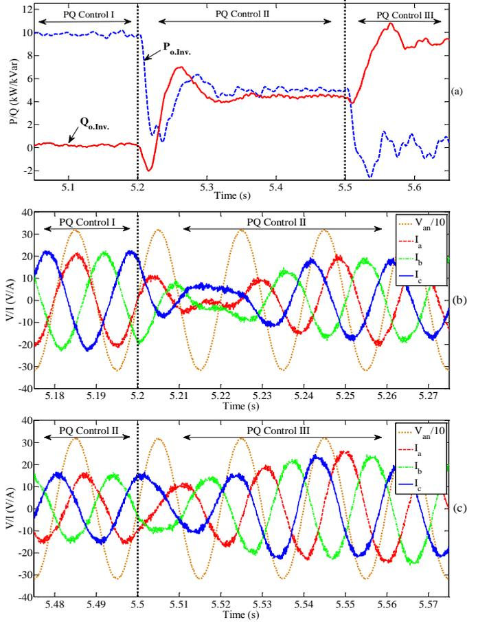
Fig. 8. Performance of the proposed controller under different balanced PQ control strategies: (a) Inverter active and reactive power, (b) Inverter current and PCC phase voltage under PQ control I and II, and (c) Inverter current and PCC phase voltage under PQ control II and III.
