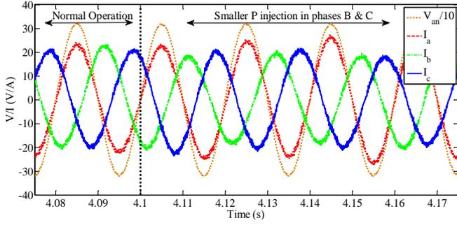
Fig. 9. Inverter output current under unbalanced active power injection
