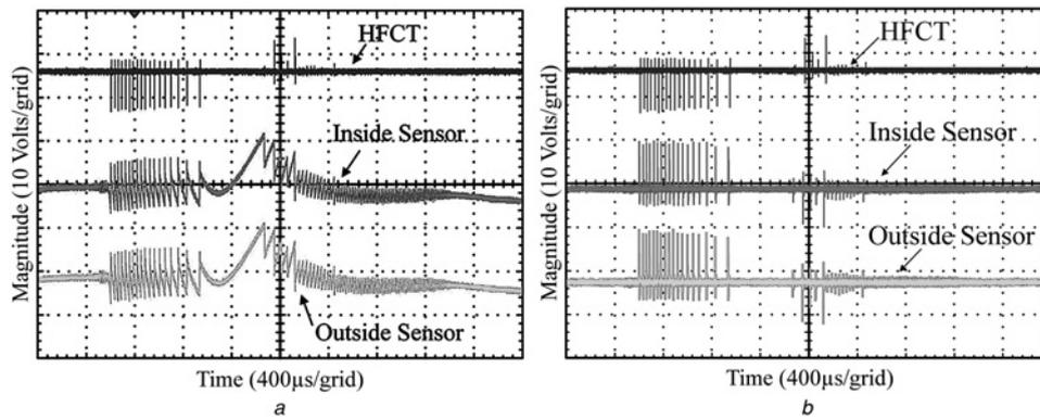
**Fig. 3** Measured PD signals from different sensors before and after filtering
