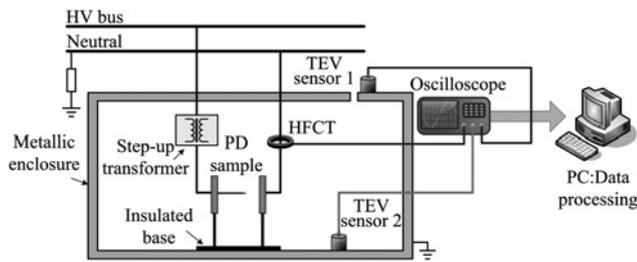
Fig. 1 Measurement setup of laboratory test
