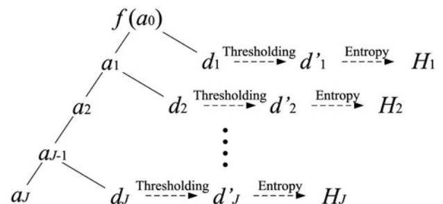
**Fig. 7** Fundamental of entropy based feature extraction
