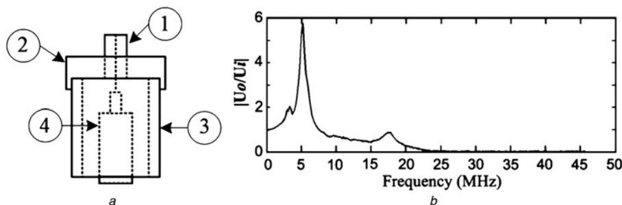
Fig. 2 Coaxial PD sensor developed for non-intrusive PD measurement
