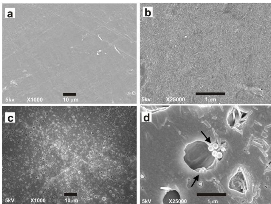
**Figure 2.** SEM images of the plain PCL film and SiNP-PCL nanocomposite film: (a, b) plain PCL film and (c, d) SiNP-PCL nanocomposite film visualized under different resolutions. Scale bars: 10  $\mu\text{m}$  for a and c; 1  $\mu\text{m}$  for b and d. Black arrows indicate the silica nanoparticles.
