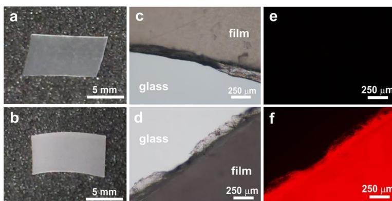
**Figure 1.** Plain PCL film and SiNP-PCL nanocomposite film: (a) Picture of plain PCL film and (b) SiNP-PCL nanocomposite film; (c, d) Bright field and (e, f) fluorescence images of plain PCL film (c, e) and SiNP-PCL nanocomposite film (d, f).
