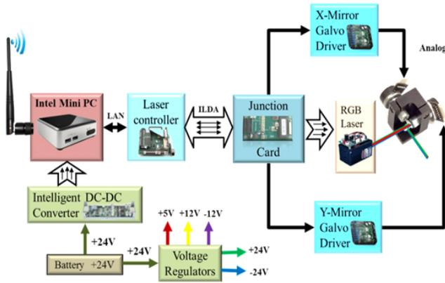
Figure 1. Laser writer main component diagram.
