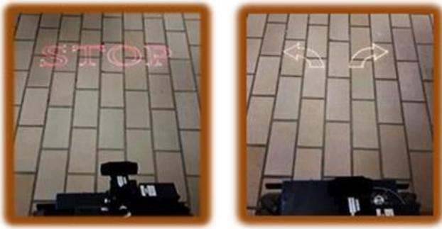
Figure 4. Projecting laser images on the floor.
