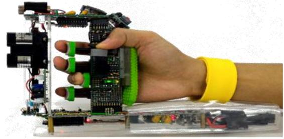
Figure 9. The first prototype of the handheld device.
