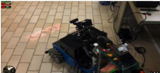
Figure 12. MAVEN projects its current status “STOP” on the floor.
