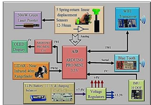
Figure 10. The handheld device hardware block diagram.
