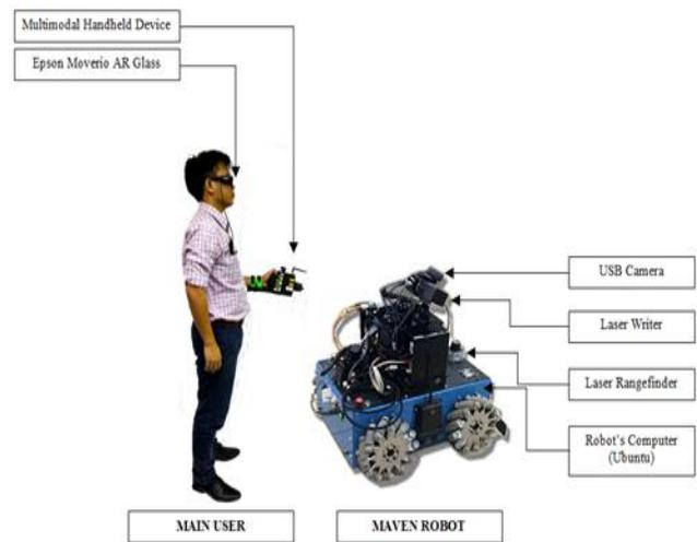
Figure 13. The implementation of the proposed human-robot framework.
