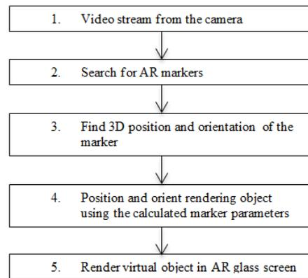
Figure 6. AR content creation using marker tracking diagram.
