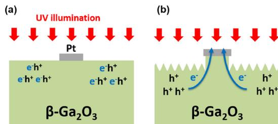
FIG. 2. Schematic illustration of the hypothesized I-MacEtch process that forms the nanoscale grooved textures: (a) Generation of electron ( $e^-$ ) and hole ( $h^+$ ) pairs in the  $\beta$ -Ga<sub>2</sub>O<sub>3</sub> region not covered with Pt by 254 nm UV illumination. (b) Diffusion of photo-excited electrons towards the Pt catalyst by the reduction of the oxidant, leaving behind excess photo-excited holes to etch  $\beta$ -Ga<sub>2</sub>O<sub>3</sub>.
