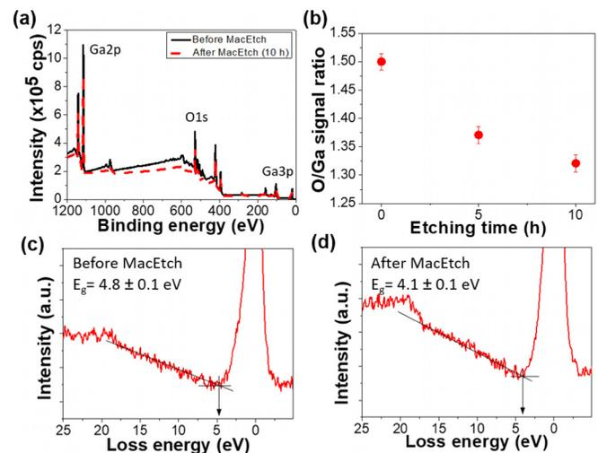
FIG. 3. XPS characterization of the  $\beta$ -Ga<sub>2</sub>O<sub>3</sub> surface before and after MacEtch: (a) XPS survey scan. (b) O/Ga ratio as a function of etching time based on O1s and Ga2p peak intensity. (c) and (d) Energy loss spectra of O1s photoelectrons for  $\beta$ -Ga<sub>2</sub>O<sub>3</sub>. The band-gap energy is extracted by the intercept of the linear extrapolation of the leading edge to the background level.
