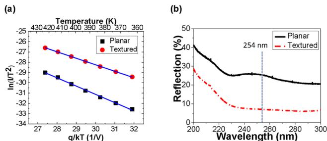
FIG. 4. (a)  $\ln(I/T^2)$  vs.  $q/kT$  plot of Pt/ $\beta\text{-Ga}_2\text{O}_3$  Schottky diodes. The SBHs of the planar and textured Schottky diodes extracted are 1.49 and 1.36, respectively. (b) Measured surface reflection spectra of  $\beta\text{-Ga}_2\text{O}_3$  before and after MacEtch texturing.
