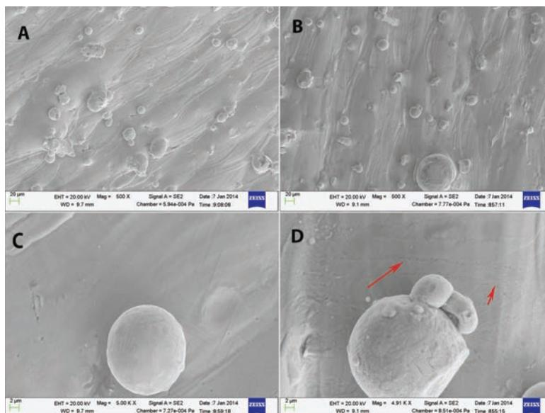
Figure 3. (A) 500x SEM of laser-sintered Co-Cr alloy (non heat-treated) (B) 500x SEM of laser-sintered (non-heat treated) (C) 5000x SEM of non heat-treated Co-Cr alloy without crevices (D) 5000x SEM of heat-treated Co-Cr alloy with crevices (arrows).
