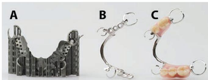
Figure 1. Stages of production for a laser sintered removable partial denture. A) Dental prosthesis directly after manufacturing, B) with support structures removed and surface polished, C) after completion (left to right). *Source: EOS GmbH*
