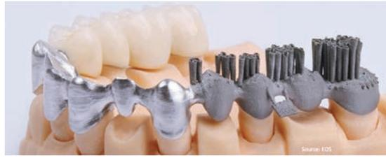
Figure 2. Dental prostheses (steps in production from left to right: with support structures, surface ready for veneer, after ceramic veneer) on a dental model. *Source: EOS GmbH*
