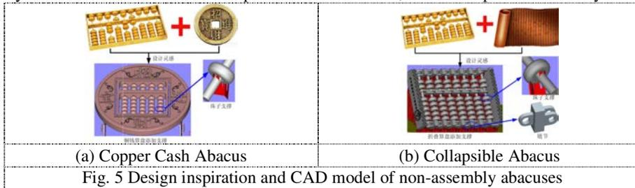
Fig. 5 Design inspiration and CAD model of non-assembly abacuses
