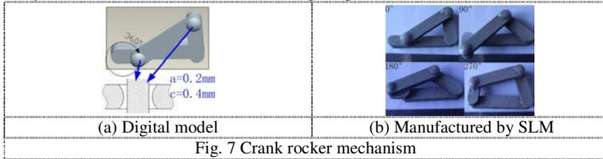
Fig. 7 Crank rocker mechanism
