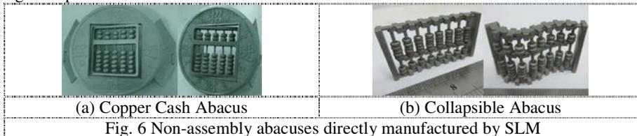
Fig. 6 Non-assembly abacuses directly manufactured by SLM
