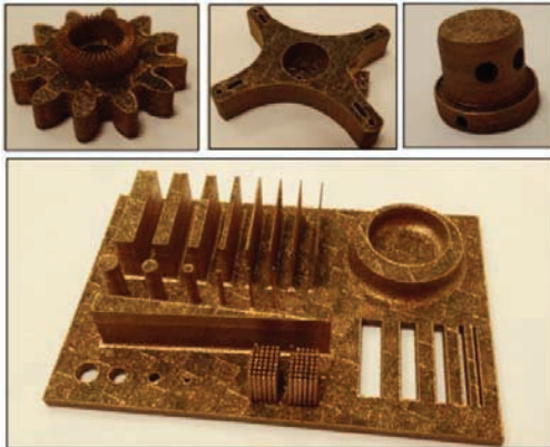
Figure 1: SLM parts produced using K220 powder
