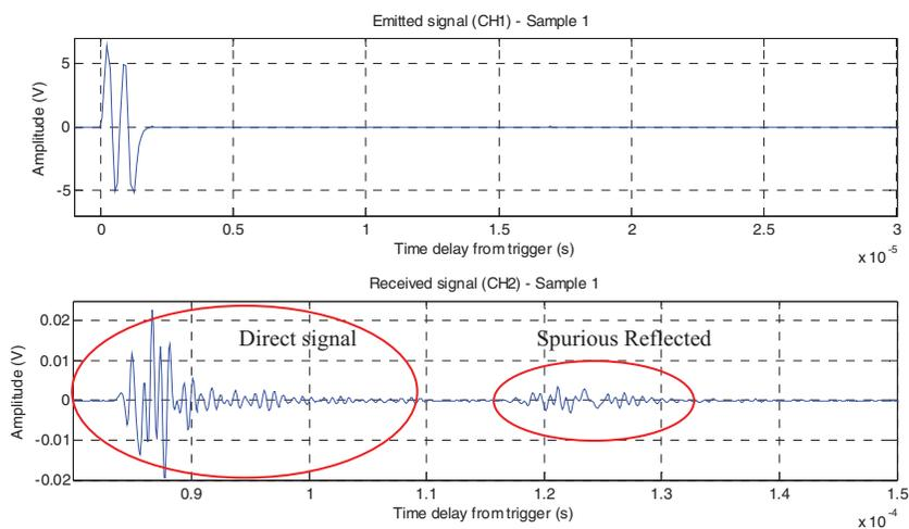
Figure 5. The applied and received signals for the measurement of the zirconia sample showing the direct arrival and a spurious reflection
