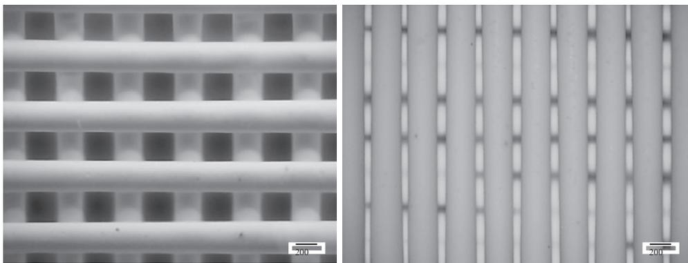
Figure 4. Microscopic images of sintered zirconia lattices with 300 and 70 microns pores
