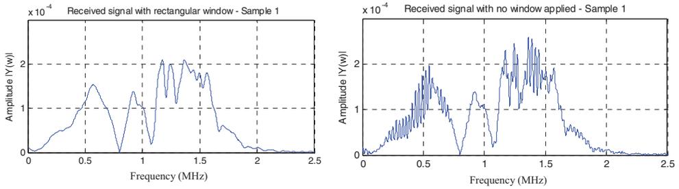
Figure 6. Frequency spectrum of the received signal with no window (right) and rectangular window applied for the Sample (left)
