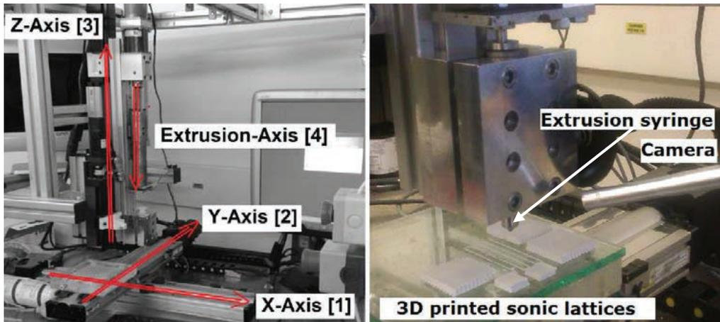
Figure 1. Experimental set up of the extrusion freeforming device
