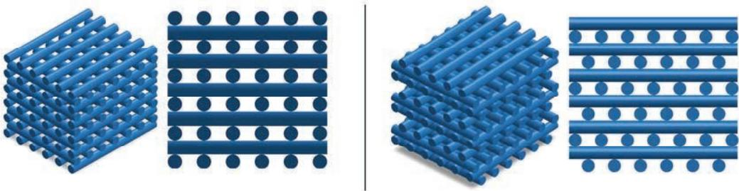
Figure 2. Different acoustic woodpile designs: normal acoustic woodpile (left), and woodpile structure with a shifted rods arrangement (right)
