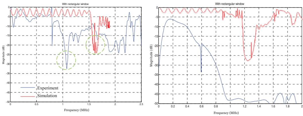
Figure 7. a) Transfer function of the normal designed zirconia sample with rectangular window applied b) transfer function of the shifted rods designed alumina sample with rectangular window
