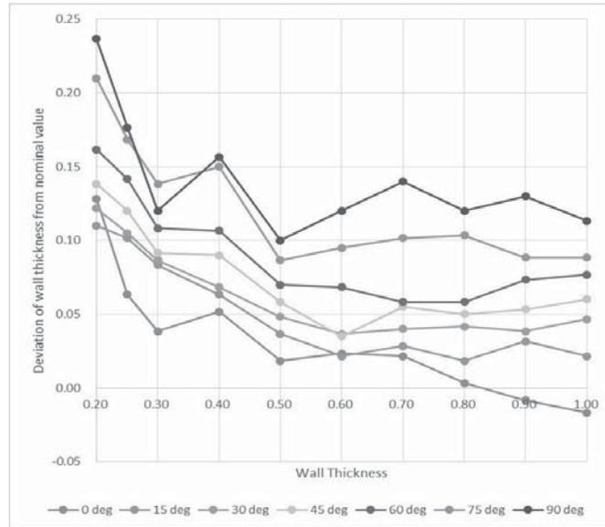
Figure 4. Deviation of wall thickness from nominal value
