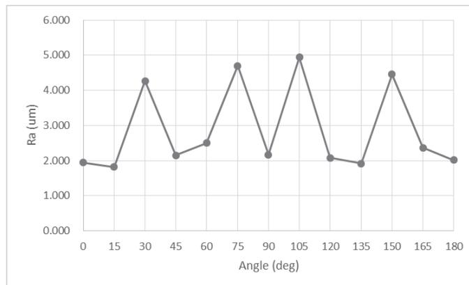
Figure 2. Effects of orientation on the surface roughness of the thin walls.
