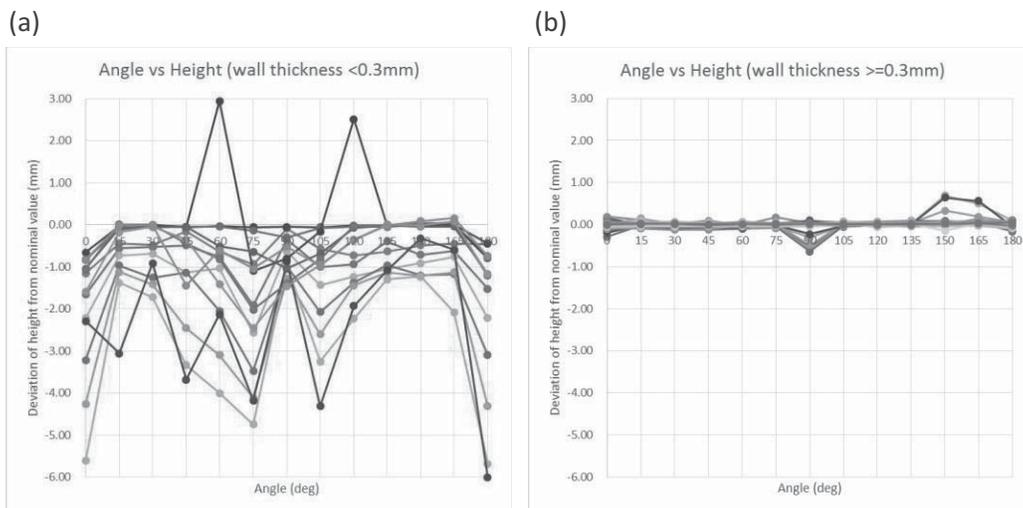
Figure 3. Deviation of height from nominal height against different angles for: (a) wall thickness < 0.3mm, (b) wall thickness  $\geq$  0.3mm
