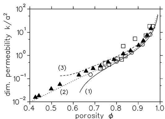
FIG. 4. The calculated dimensionless permeability  $k/a^2$  as a function of porosity (black triangles). Open squares and circles show the experimental results for fibrous filters [5] and compressed fiber mats [3,5], respectively. Curve (1) is the analytical result for cubic lattice given in Ref. [5], curve (2) is the numerical result for an fcc lattice from Ref. [19], and curve (3) shows the result of a fit with the Kozeny-Carman relation, Eq. (3).
