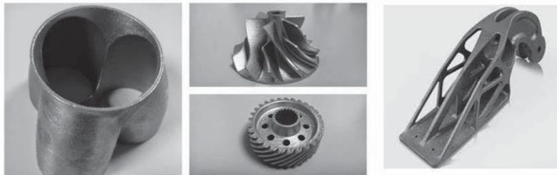
Figure 4. Automobile and Aerospace part produced by SLM process [Source: <http://www.tctmagazine.com/3D-printing-news/slm-solutions-and-eads-partner>]
