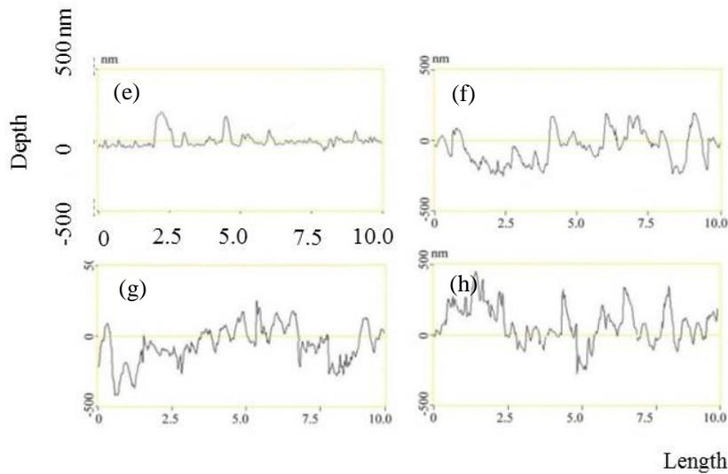
Fig. 3 Profiles of topographical evolution on AZ31B Mg alloy surfaces at laser scanning number of: (a) and (e) 5; (b) and (f) 10; (c) and (g) 30; (d) and (h) 50. Laser pulse energy is 30  $\mu\text{J}$  and scanning speed is 50 mm/s.
