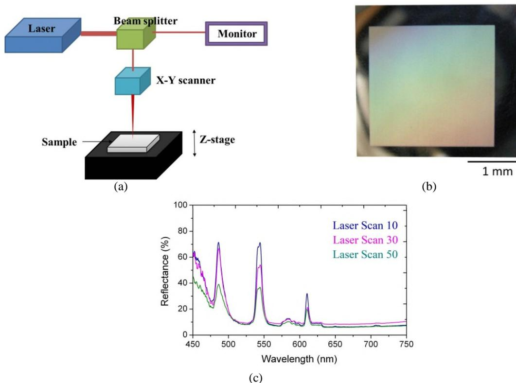
Fig. 1 (a) Femtosecond laser setup used for writing large-area structured color on AZ31B Mg alloy surface; (b) Photographs of typical iridescent effect on the irradiated surface by femtosecond laser scanning 30 times at pulse energy of 30  $\mu$ J and speed of 50 mm/s; (c) Reflectance of laser-irradiated surfaces at laser
