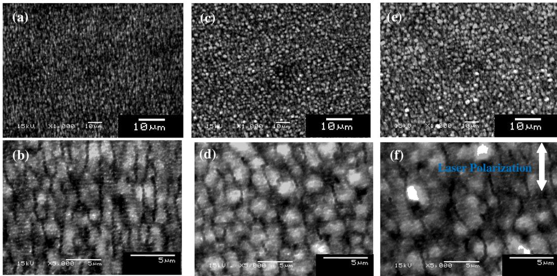
Fig. 2 Morphological evolution of AZ31B Mg alloy surfaces at laser scanning number of: (a)-(b) 10, (b) magnified image for (a); (c)-(d) 30, (d) magnified image for (c); (e)-(f) 50, (f) magnified image for (e). Laser pulse energy is 30  $\mu$ J and scanning speed is 50 mm/s.
