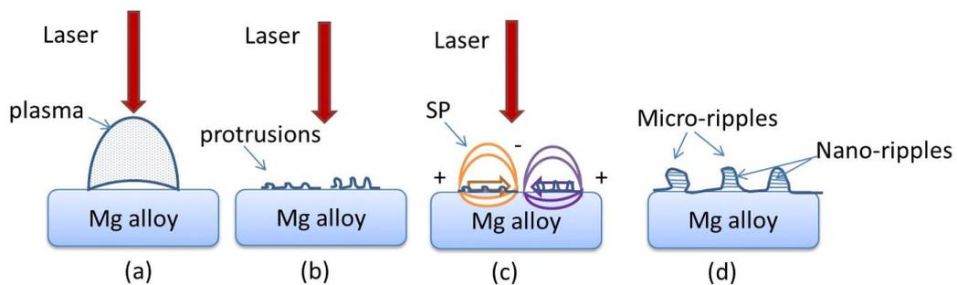
Fig. 4 Schematic representation for the formation of laser-induced ripples on AZ31B Mg alloy during femtosecond laser irradiation: (a) surface absorption, ejected species and plasma; (b) nano-protrusions; (c) developed nano-protrusions and excited surface plasmons (SP); (d) micro-ripples and nano-ripples generation.
