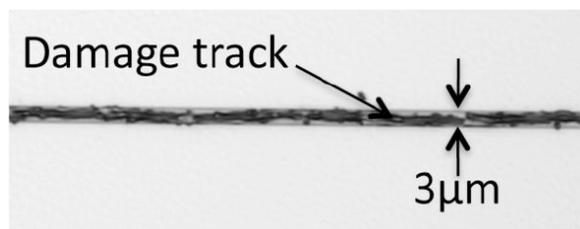
Fig 1. “fiber fuse” damage in a  $3\mu\text{m}$  wide  $\text{Ge}_{11.5}\text{As}_{24}\text{Se}_{64.5}$  rib waveguide without  $\text{Al}_2\text{O}_3$  coating exposed to CW power around  $40\text{mW}$ . The track extends over a distance of about  $1\text{cm}$  in this case and appears to originate at a defect in the waveguide. The molten damage snakes along the waveguide back to the entrance surface
