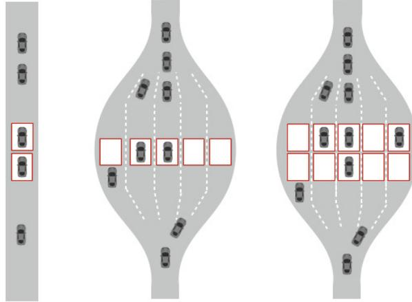
Figure 1: Schematic illustration of 3 types of bottleneck expansions: serial ( $m = 2$ ); parallel ( $n = 5$ ); and combination ( $m = 2, n = 5$ ). Note that direction of travel is upwards
