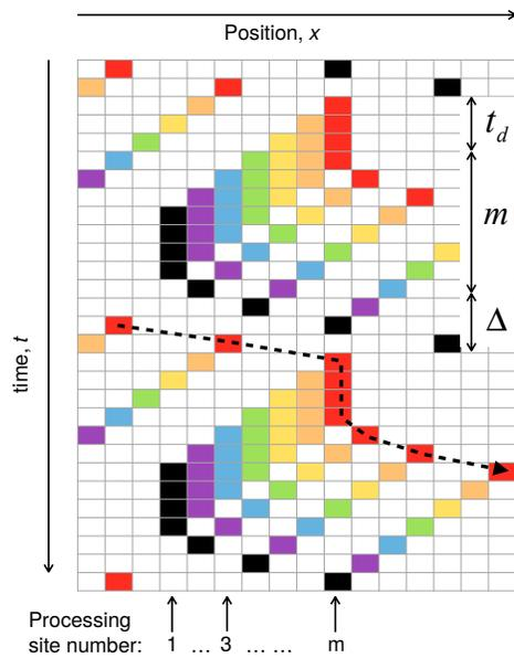
Figure A.9: A plot of the space-time trajectories of vehicles moving through a serial bottleneck at critical density. The parameters of the simulation are:  $m = 7$ ,  $t_d = 3$ , and  $v_m = 4$ . Note that the different colors are used to differentiate each vehicle, and the repeated colors do not represent the same vehicle. The dotted line indicates the trajectory of one of these vehicles.
