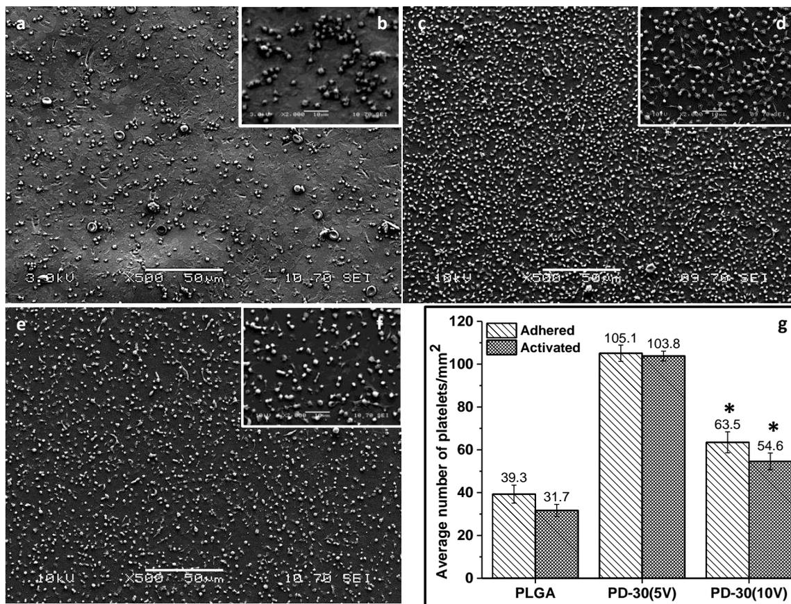
**Figure 3.** SEM photomicrographs (a-f) of the adhered platelets over the surface of PLGA (a, b) and electrocured PD-30 at 5V (c, d) and 10V (e, f), and the quantitative analysis of the adhered and activated platelets over different bioadhesive surface (g). \*Significant at  $p < 0.05$  among the similar comparison groups (adhered/activated); a, c, e: low magnification and b, d, f: high magnification SEM photomicrographs
