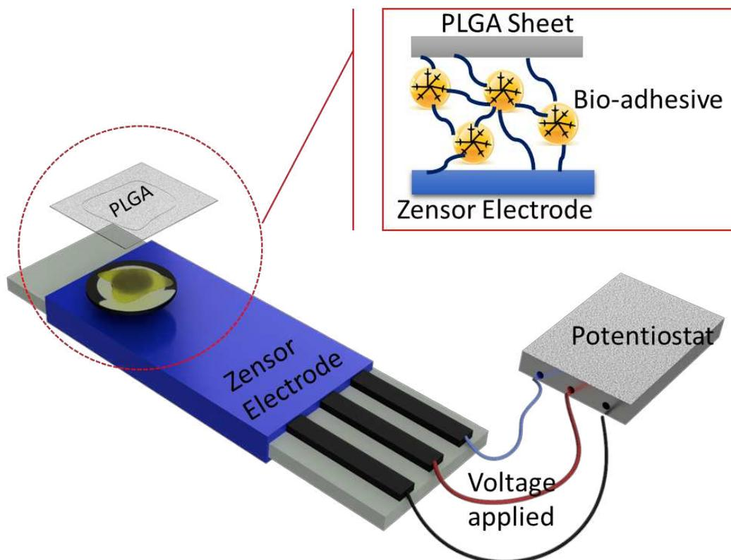
**Figure 1.** A schematic presentation showing the set up for the electrical activation of bioadhesive using Zensor electrode
