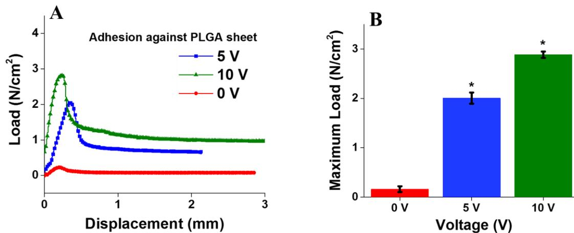
**Figure 2.** Lap-shear adhesion strength t. Load vs displacement curve of electrocured PD-30 bioadhesives using 1X PBS at a concentration of 50 wt% (A), and a comparison of maximum load values obtained across all tested voltages (0V, 5V, and 10V) after 10 minutes of electrical activation (B). \*Significant at  $p < 0.05$ .
