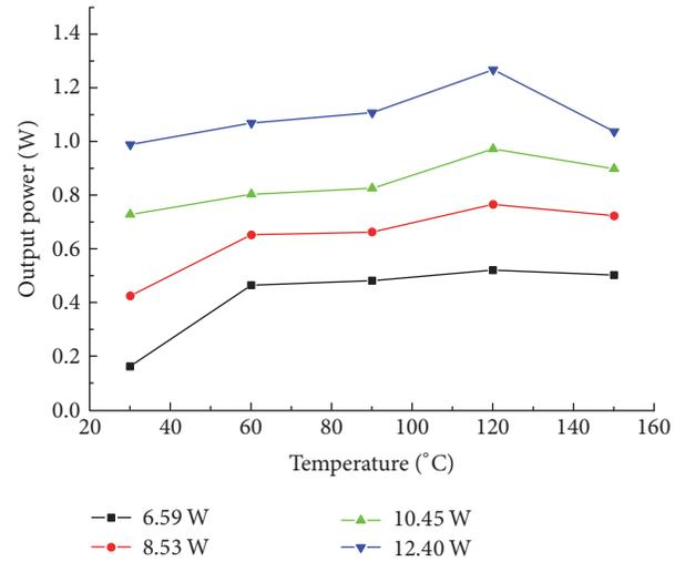
FIGURE 4: The idler output power with temperature tuning under different incident pump power.
