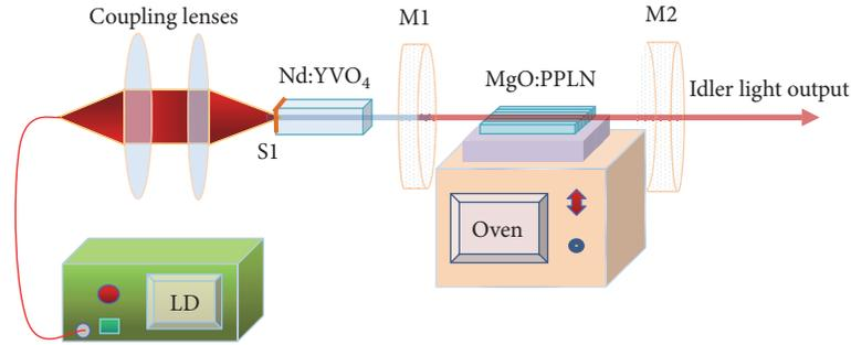
FIGURE 1: Schematic diagram of LD end-pumped intracavity singly resonant optical parametric oscillator setup.
