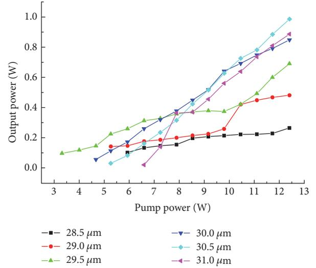
FIGURE 3: The idler output power versus incident pump power with different domain period ( $T = 30^\circ\text{C}$ ).
