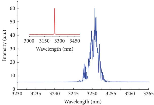
FIGURE 5: The idler spectrum of MgO:PPLN crystal at the temperature of 120°C and the grating period of 30.5  $\mu\text{m}$ .
