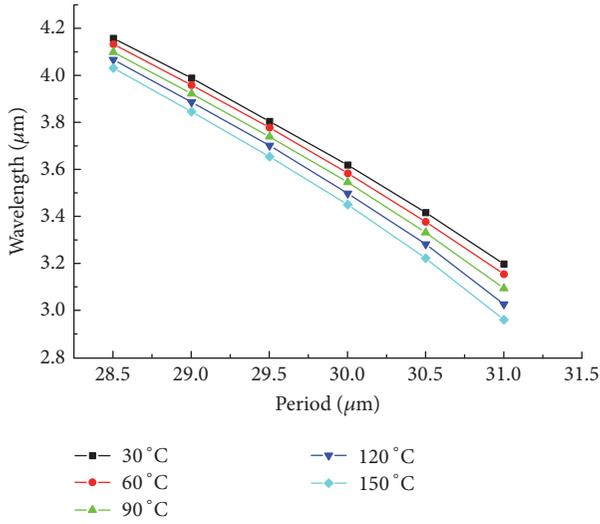
FIGURE 2: The tuning curves of the SR-OPO system versus the grating period of the MgO:PPLN crystal at different controlled temperature value.
