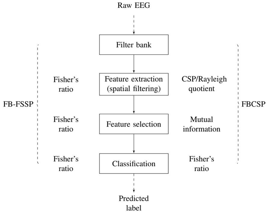
Fig. 1. The flow chart of the EEG signal processing procedures in FB-FSSP and FBCSP.
