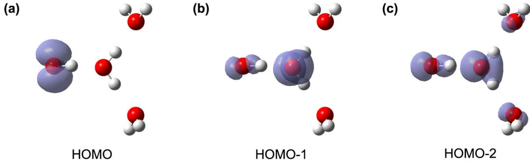
**Figure 4.** Orbital densities of the (a) HOMO, (b) HOMO–1, and (c) HOMO–2 of  $(\text{H}_2\text{O})_4$ . Note the orthogonal directions of the dominant orbital densities of the different molecular orbitals, which suggests that their coherent superposition would give rise to a periodic reorientation of the hole density in the  $(\text{H}_2\text{O})_4^+$  ion.
