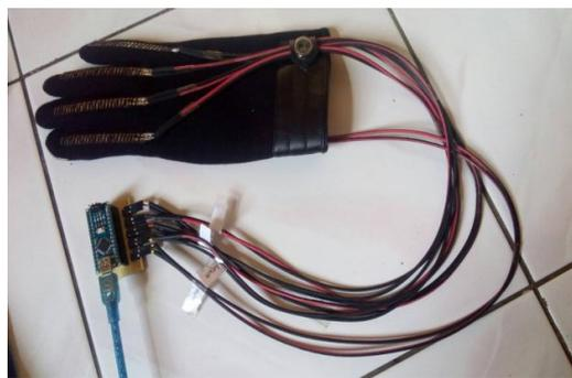
**Figure 4.** Glove, PCB and Arduino installation.
