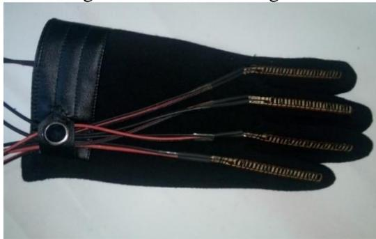
**Figure 3.** Glove with flex sensors.
