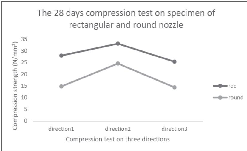
Figure 5: 14-days and 28-days Compression Test Result
