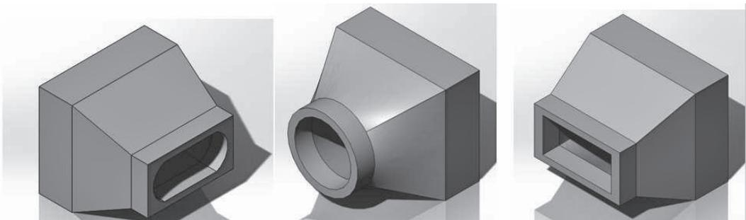
Figure 2: CAD Models for Different Nozzle Outlets
