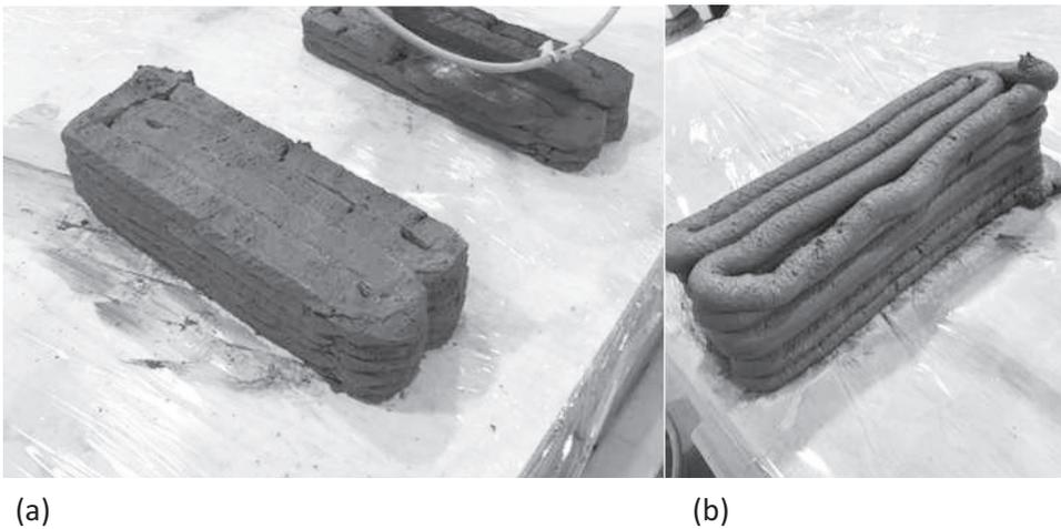
*Figure 3: Printing Test with Different Nozzles*
