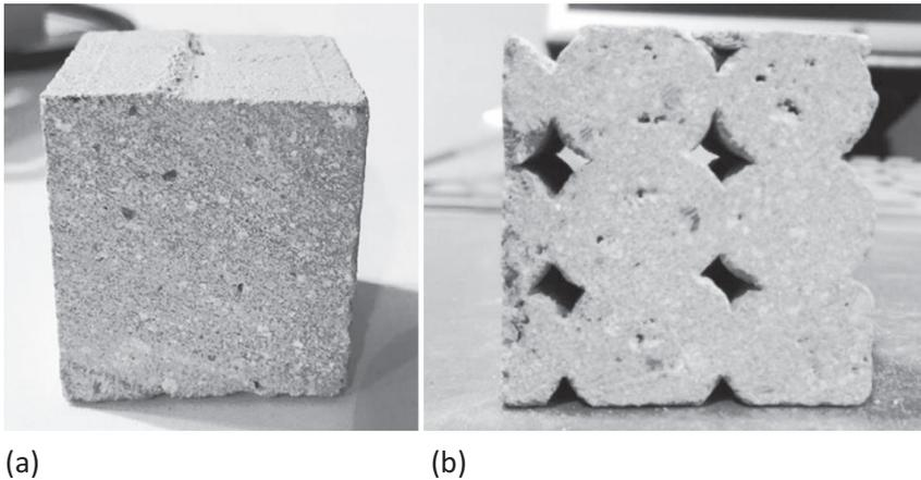
Figure 4: Cross-Sectional View of Specimen Printed with Different Nozzles
