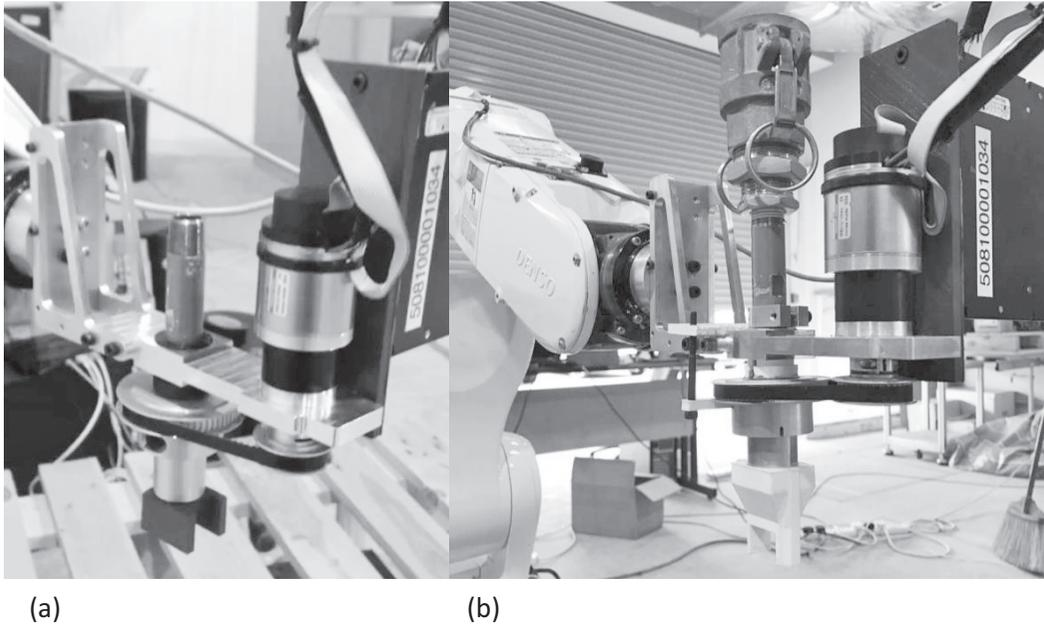
Figure 1: Mechatronic Nozzle Assembly and DENSO Robotic Arm
