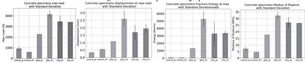
Figure 3: Key results of the load displacement graph
