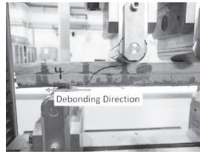
(b): Shear crack in FRP reinforced beams
