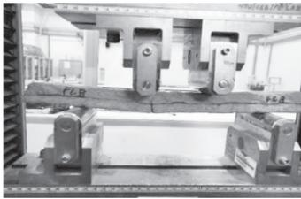
(a): Flexural crack in control beam
