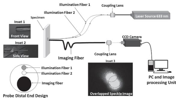
Figure 4. Proposed optical probe configuration for front view and side view ASC experiments.
