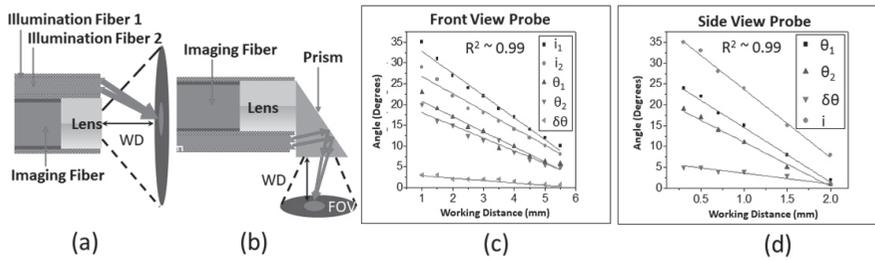
Figure 3. Shows the proposed design for the (a) front view and (b) side view ASC probe. Relationship between the fiber cleaving angle ( $i$ ) and the illumination angle ( $\theta$ ) required for the (c) front view ASC and the (d) side view ASC experiments.
