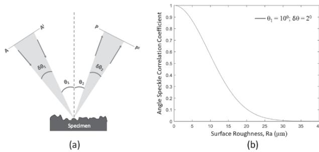
Figure 1. (a) The geometric arrangement for Angular Speckle Correlation (ASC) experiments and the theoretical plot depicting the relationship between ASC and average surface roughness, Ra, for  $\theta_1 = 10^\circ$  and  $\delta\theta [\theta_2 - \theta_1] = 2^\circ$  is shown in (b).
