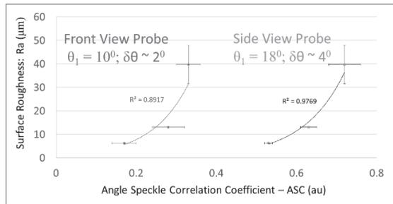
Figure 5. ASC measured using the front view and the side view probe compared with the average surface roughness, Ra, measured using the Keyence optical profiler (VR-3000).
