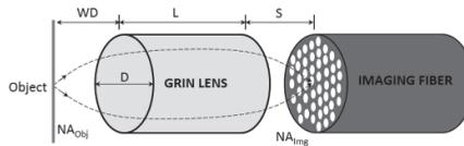
Figure 2. Schematic diagram of a GRIN lensed speckle imaging system.
