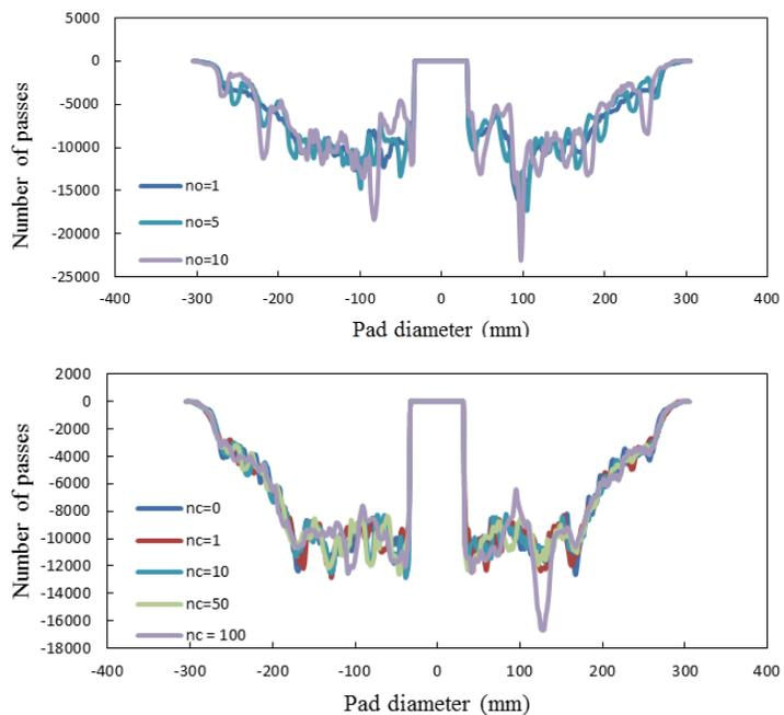
Fig. 2. Effect of the oscillation speed (strokes/min) and the rotational speed (rpm) of the conditioner on the pad wear shape.
