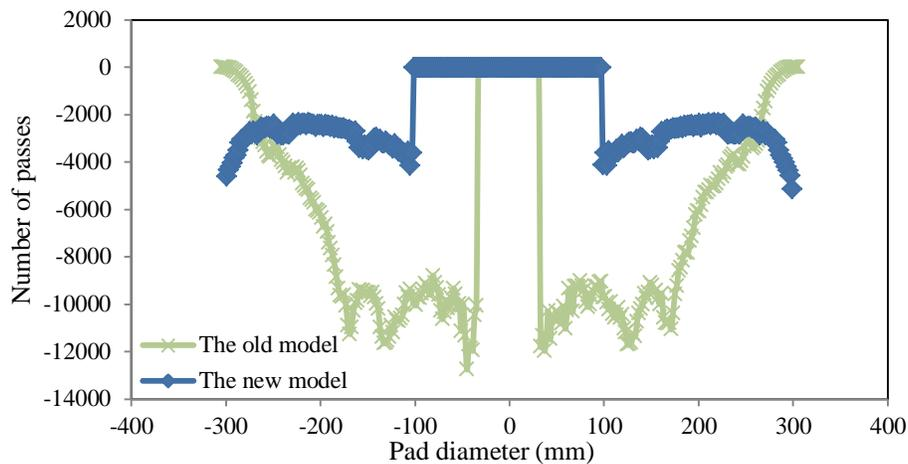
Fig.5. The pad wear shapes of the new model and the old model.
