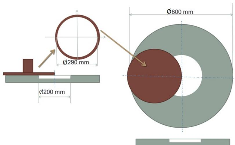
Fig.4. The new conditioner and pad in the new model.
