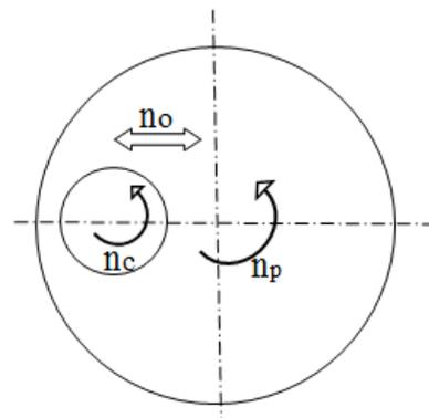
Fig. 1. Schematic representation of a conditioning process in polishing.
