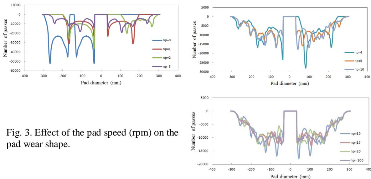
Fig. 3. Effect of the pad speed (rpm) on the pad wear shape.
