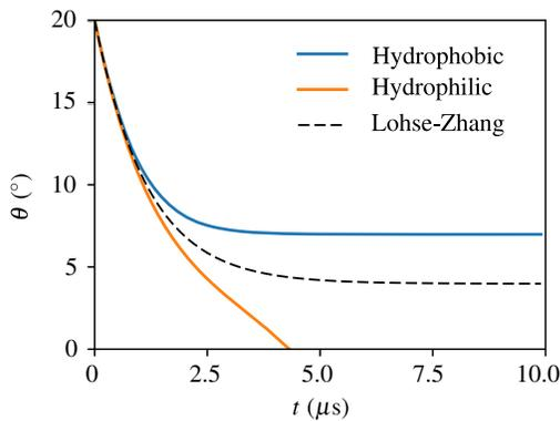
FIG. 2. Dynamical response of a nanobubble with initial footprint radius  $L = 100 \text{ nm}$  and initial contact angle  $\theta = 20^\circ$  for a liquid with far-field concentration  $c_\infty = 2c_{\text{sat}}$ . The curves are for hydrophobic ( $\phi_0/k_B T = -2$ , blue line) and hydrophilic ( $\phi_0/k_B T = 2$ , orange) substrates in the current theory, and the equivalent condition ( $\zeta = 1$ ) in the Lohse-Zhang theory is shown as a black dashed line.
