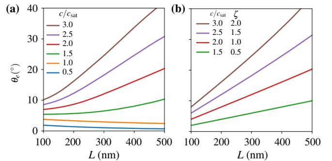
FIG. 3. Equilibrium contact angles of nanobubbles in liquids with varying  $c_\infty/c_{\text{sat}}$  in the (a) present theory and (b) Lohse-Zhang theory. Each curve represents one value of dissolved gas concentration  $c_\infty/c_{\text{sat}}$  in the liquid. The substrate is assumed hydrophobic ( $\phi_0/k_B T = -2$ ). In the Lohse-Zhang model, nanobubbles are stable only in supersaturated liquid ( $c/c_{\text{sat}} > 1$  or  $\zeta > 0$ ).
