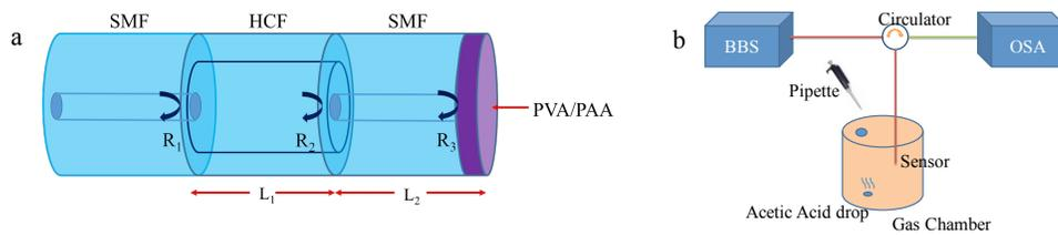
Figure 1 a. Experiment setup for hazardous gas sensing b. Schematic diagram of the FPI sensor
