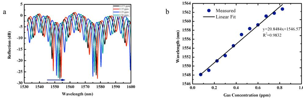
Figure 3 a. Reflection spectra of the FPI exposed to acetic acid vapor b. Wavelength shift upon the acetic acid vapor concentration
