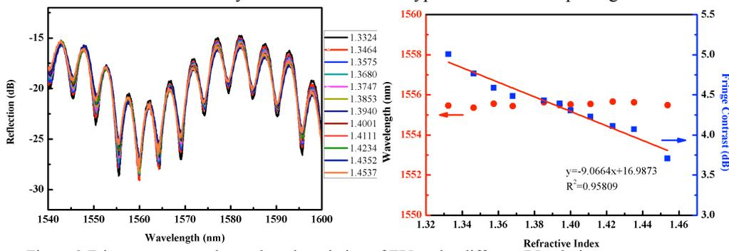
Figure 2 Fringe contrast and wavelength variation of FPI under different RI solutions
