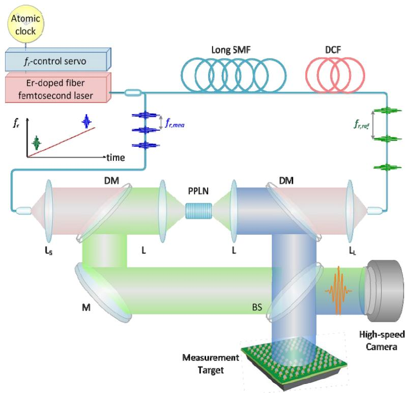
Figure 1. Low-coherence scanning interferometer using femtosecond pulses in the time domain for 3-D profilometry of microelectronic step-structures. Abbreviations are; SMF: single-mode fiber, DCF: dispersion compensating fiber, DM: dichroic mirror, PPLN: periodically poled lithium niobate.
