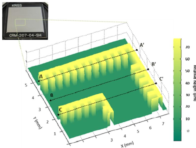
Figure 3. Measurement of high step-structures by low-coherence interferometer. Reconstructed 3-D profile showing step heights of  $\sim 69.6 \mu\text{m}$ .
