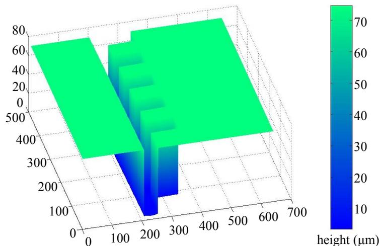
Figure 5. Measurement of high step-structures using frequency-comb-referenced multiple wavelengths. Reconstructed 3D surface profile of the standard step-specimen.
