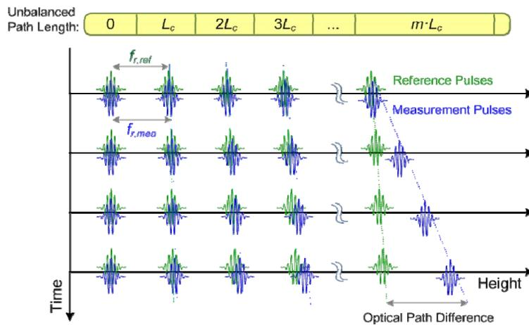
Figure 2. Conceptual diagram of relative scanning effect between the reference and measurement pulses at unequal-path interferometry.
