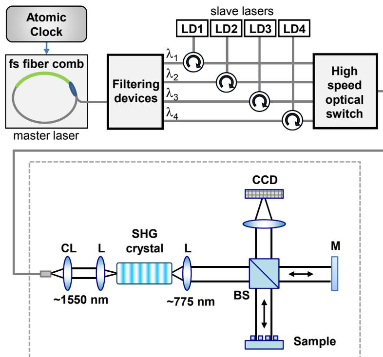
Figure 4. Frequency-comb-referenced multi-wavelength interferometer for large step-height measurement.
