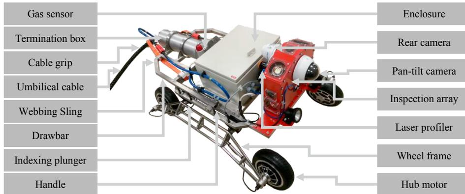
Fig. 2. Compact Mobile Robot for Sewer Inspection.
