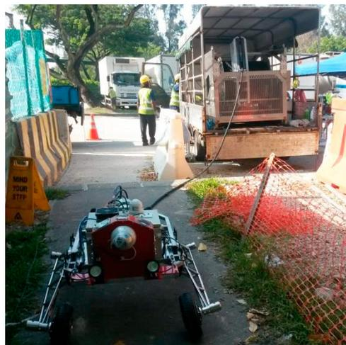
Fig. 6. Robotic Platform Attached to Umbilical-Winch System
