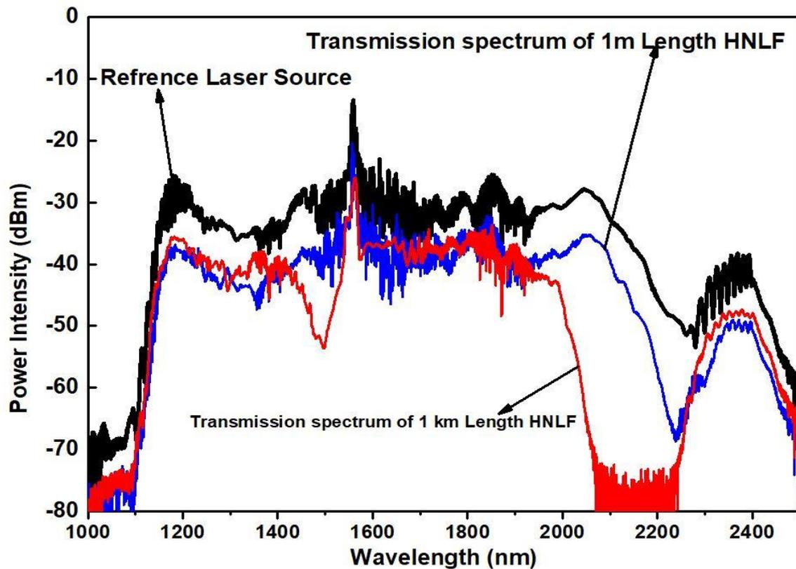
Figure 4. 12 Measured transmission spectrum from 1-km and 100-cm-long DS-HNLF over a wavelength range of 1125 nm to 2475 nm.
