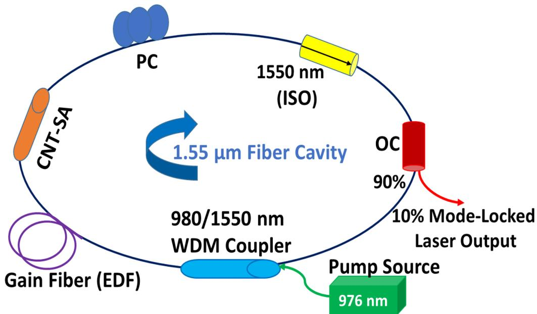
Figure 3. 3 Experimental setup of passively mode-locked fibre laser incorporating CNT-SA.
