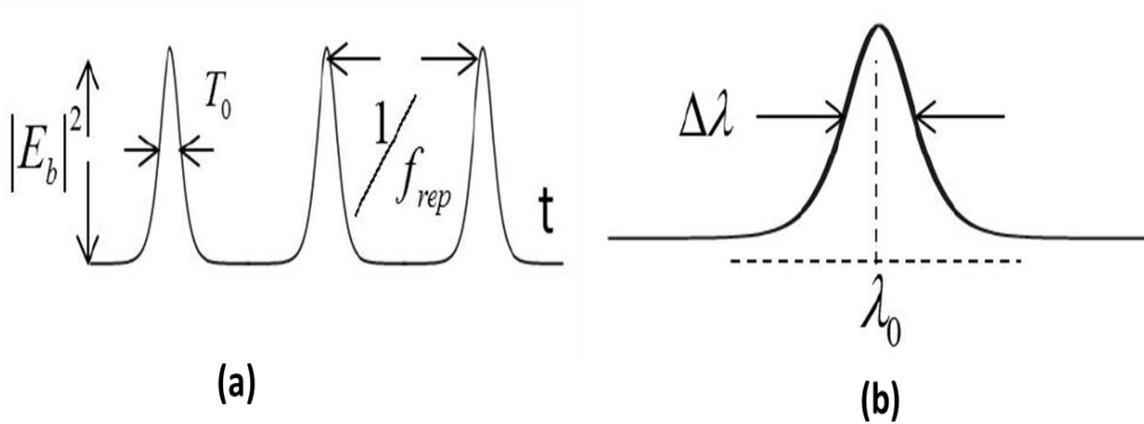
Figure 3.2 Mode-locked fibre laser pulse key performance parameters: (a) mode-locked laser pulse output in time-domain, (b) mode-locked laser pulse output in frequency-domain.
