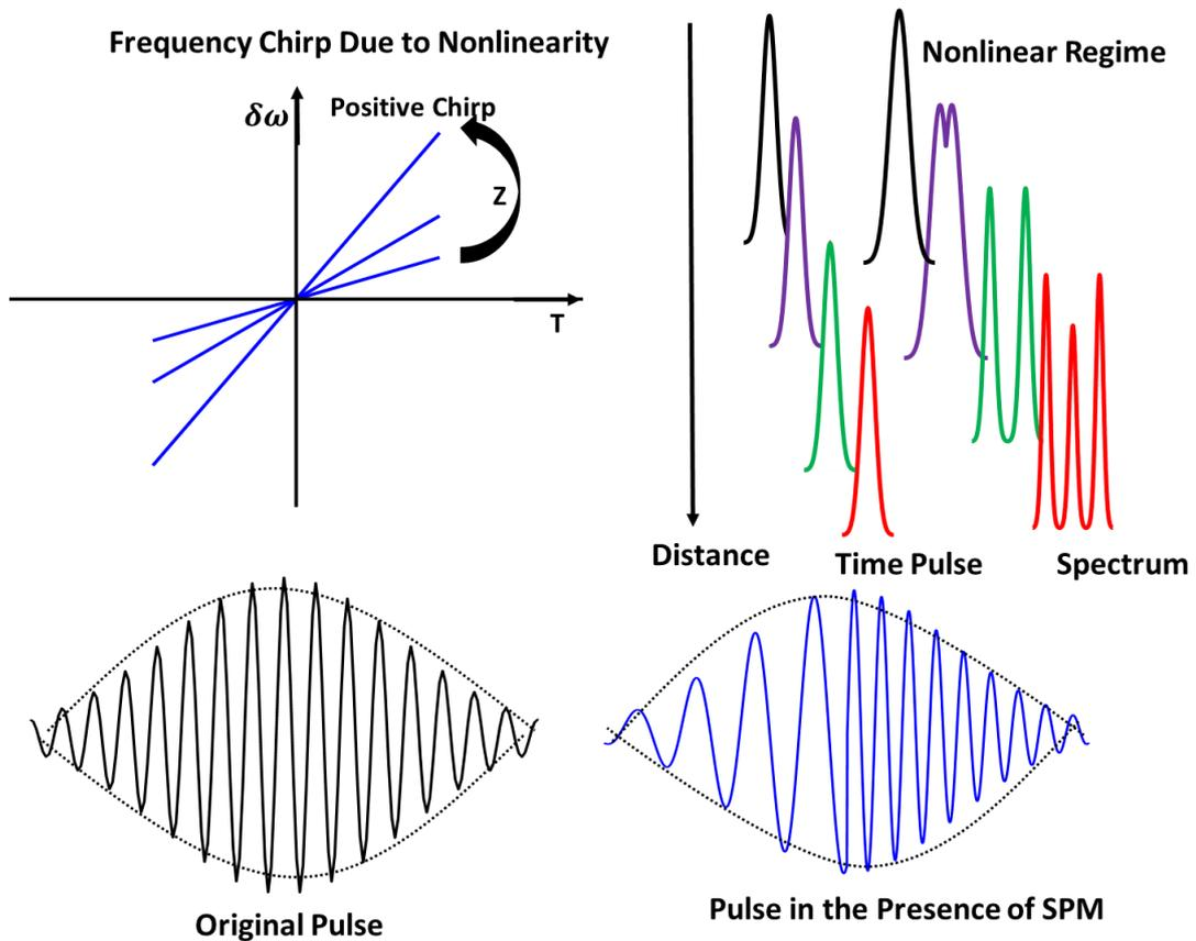
Figure 2. 14 Schematic illustration of frequency chirping phenomena and spectral broadening phenomena of pulse in nonlinearity regime [59].
