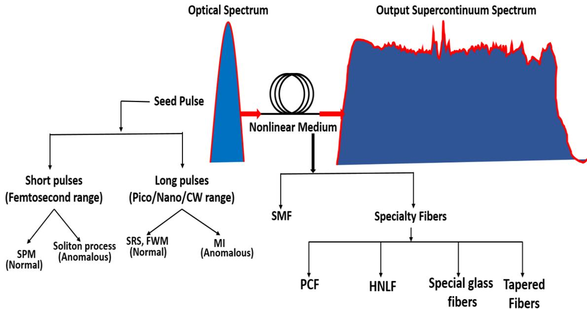
Figure 2. 10 Schematic illustration of SC generation process.
