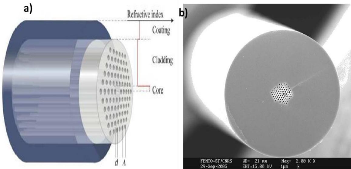
Figure 4. 1 Typical schematic of solid-core PCF [107], (b) Solid-core PCF that used for SC generation for the first time [108].
