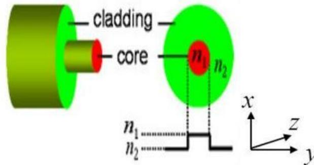
Figure 2. 11 Structural representation of optical fibre and its refractive step index profile. [58]
