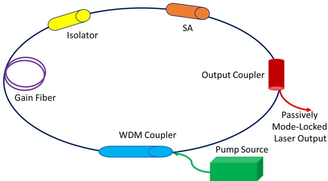
Figure 2. 8 Schematic of passively mode-locked fibre laser ring cavity; SA: saturable absorber, WDM: wavelength-division-multiplexing.
