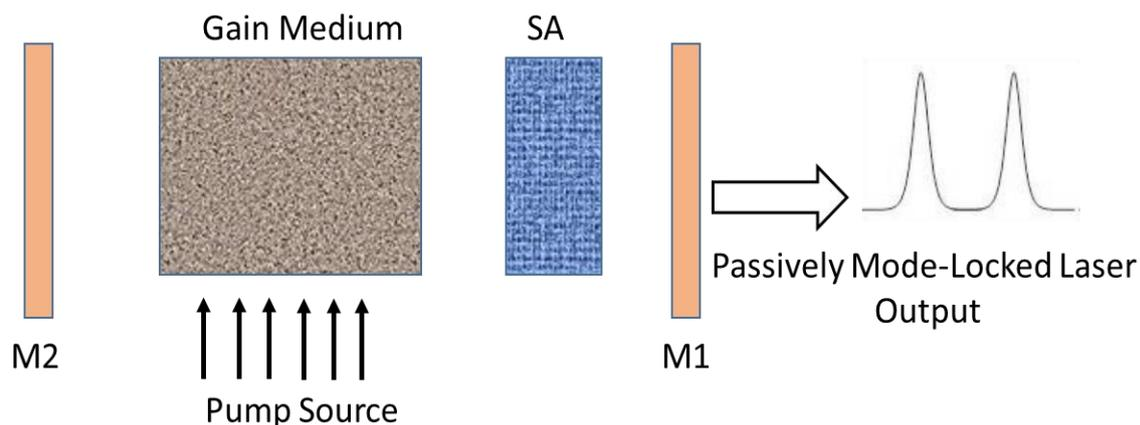
Figure 2. 7 Schematic of the passively mode-locked laser; M1: partial transmission mirror, M2: Mirror, SA: saturable absorber.
