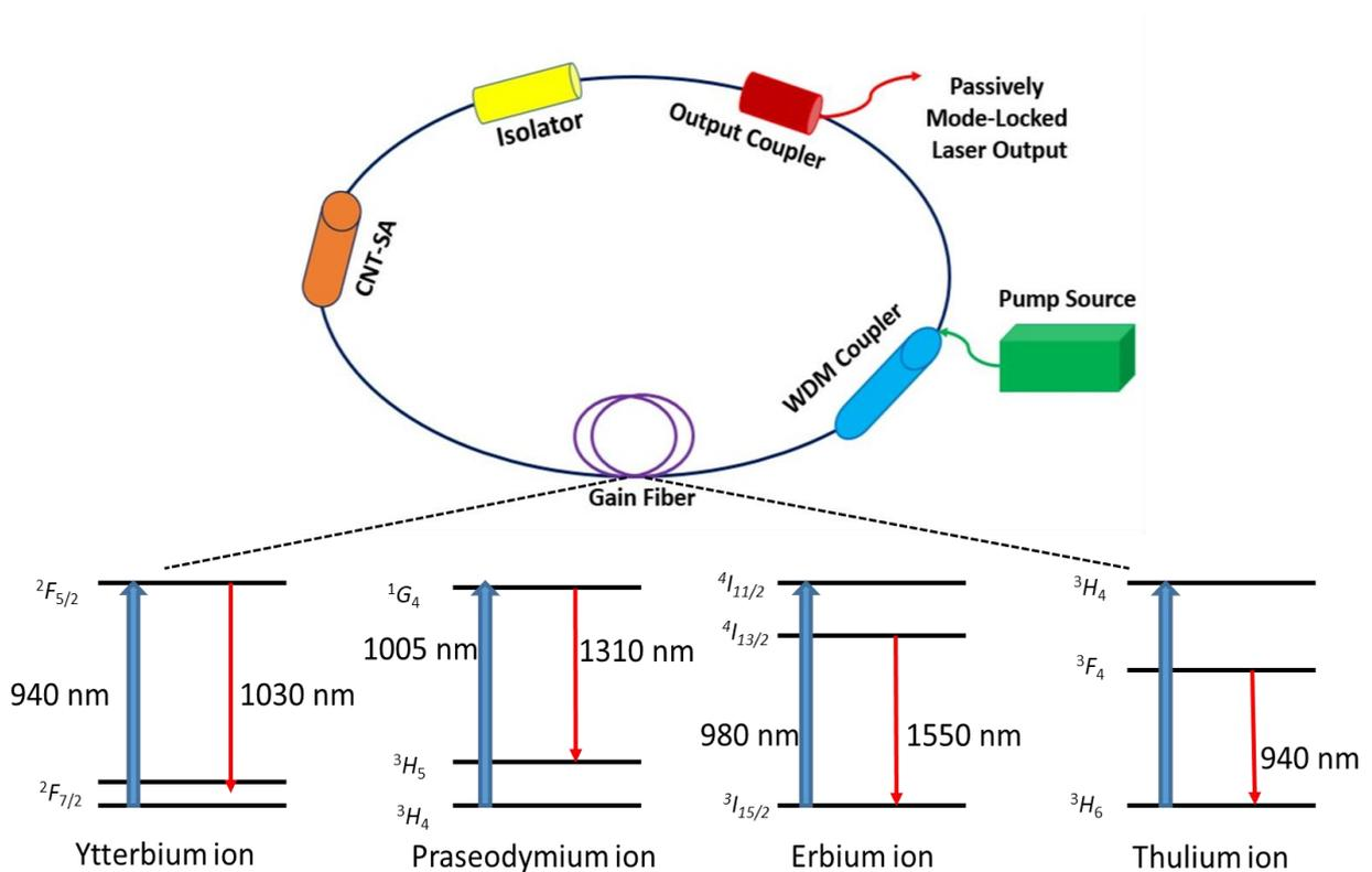
Figure 3 .1 Schematic of CNT-SA based passively mode-locked fibre lasers operating at different center wavelengths incorporating different gain fibres.
