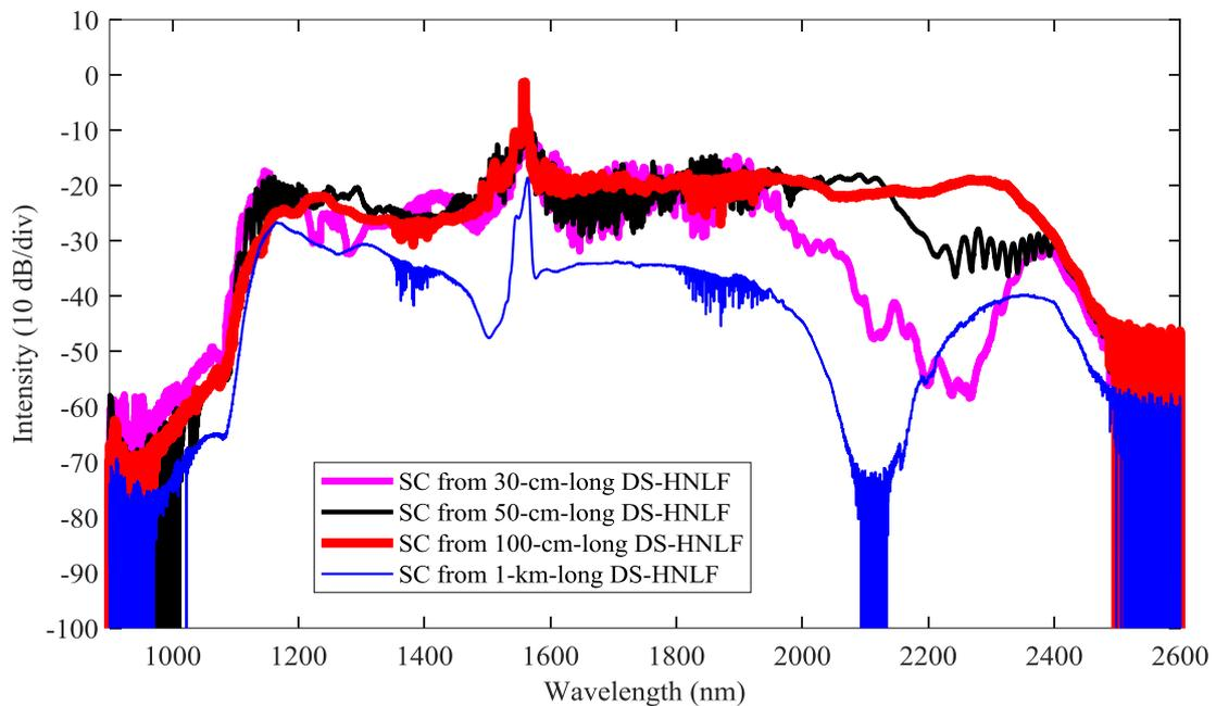
Figure 4. 13 SC spectrum from 30-cm, 50-cm, 100-cm and 1-km-length HNLF at 20 dBm input pulse power
