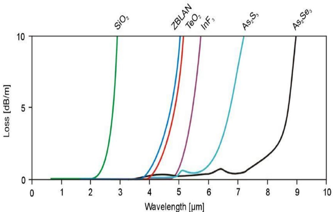
Figure 5. 1 Transmission curves for different optical fibres used for SC mid-IR SC generation [142].
