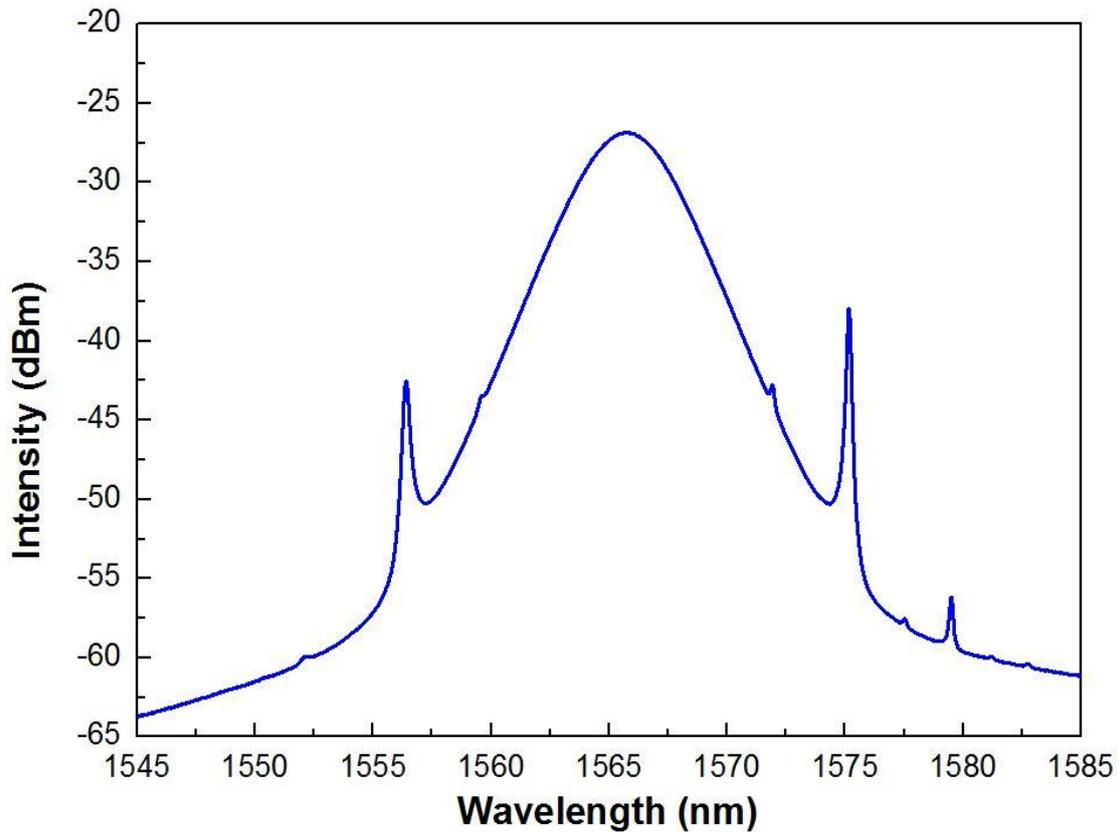
Figure 3. 6 Output spectrum of mode-locked laser pulse.
