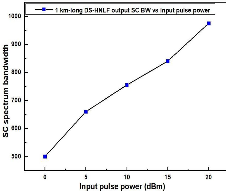
Figure 4. 7 SC spectrum bandwidth variation with respect to input pulse power variation.
