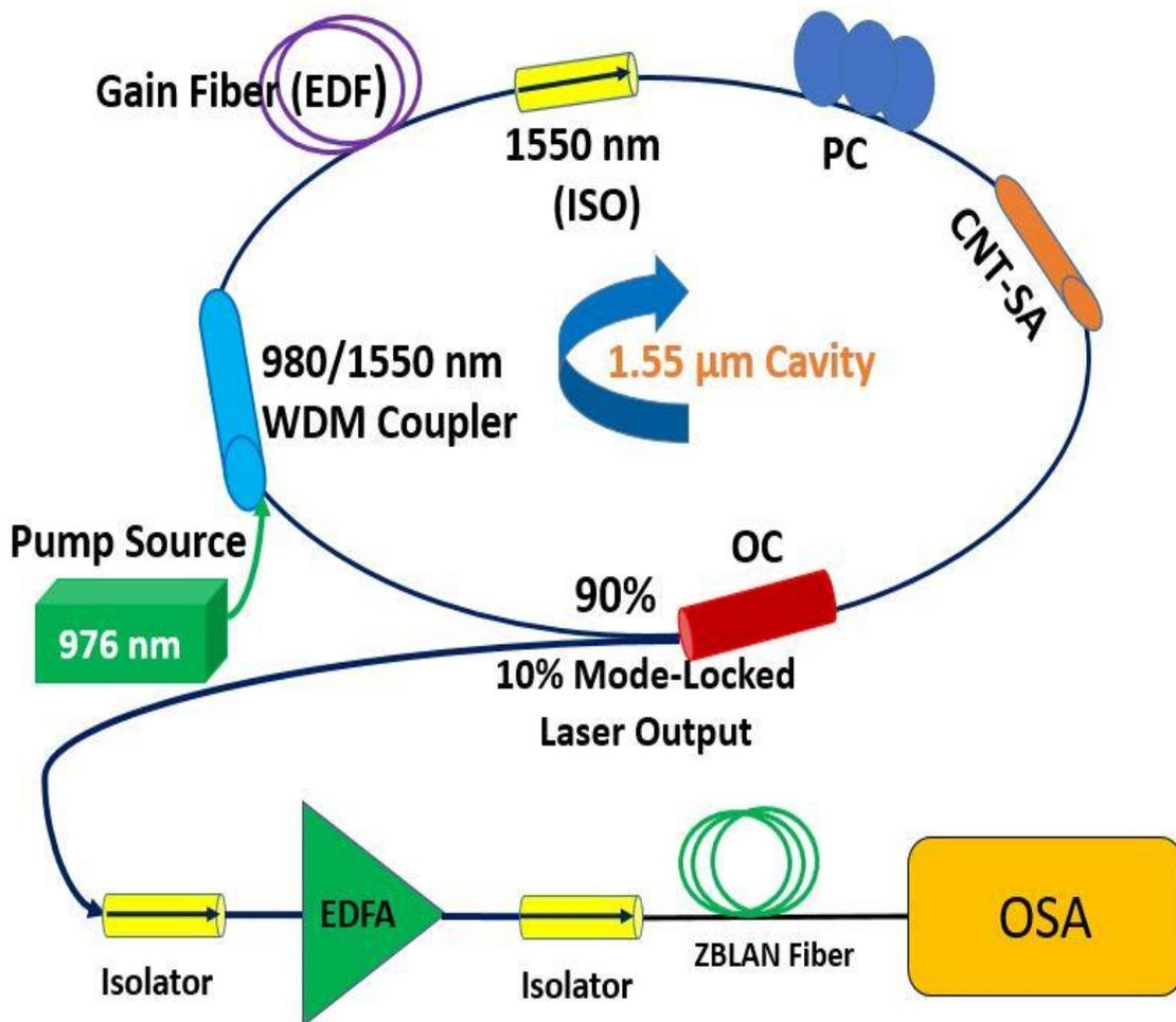
Figure 5. 2 Experimental setup of SC generation from a ZBLAN fibre using passively mode-locked fibre laser.
