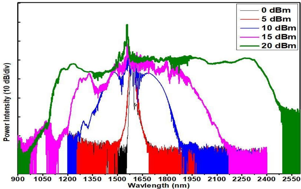
Figure 4. 10 Output SC spectral variation from 100-cm-long DS-HNLF for different input powers.
