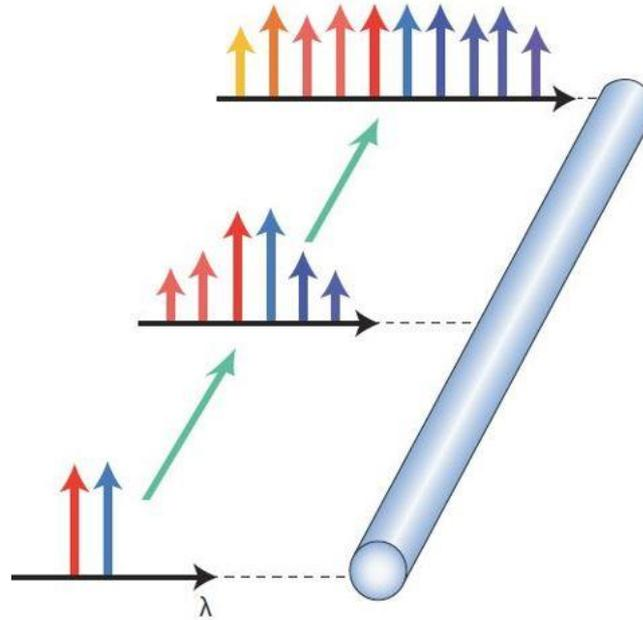
Figure 2. 16 Schematic illustration of new frequency generation in HNLF through FWM phenomena [65].
