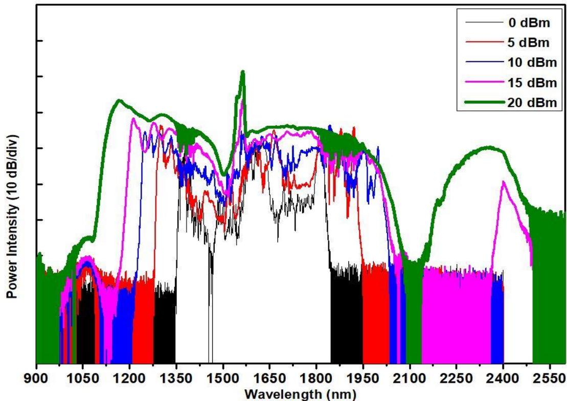
Figure 4. 6 SC spectrum output from DS-HNLF for different input pulse powers.
