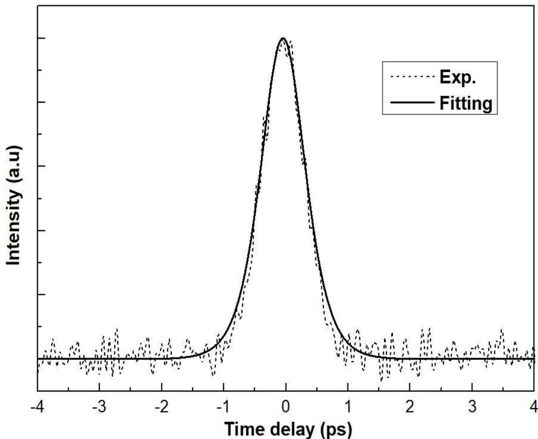
Figure 3 7 Autocorrelation trace of passively mode-locked fibre laser pulses.
