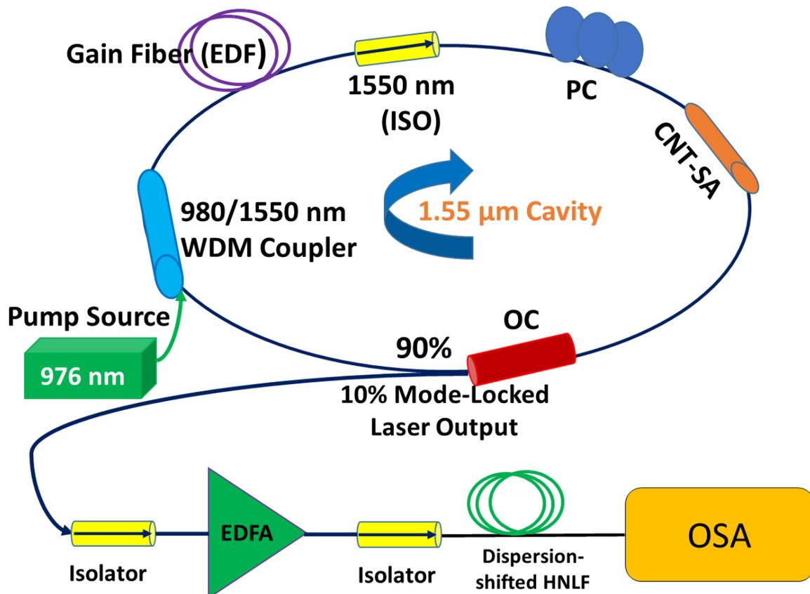
Figure 4. 5 Experimental setup of SC generation from a HNLf using passively mode-locked fibre laser.
