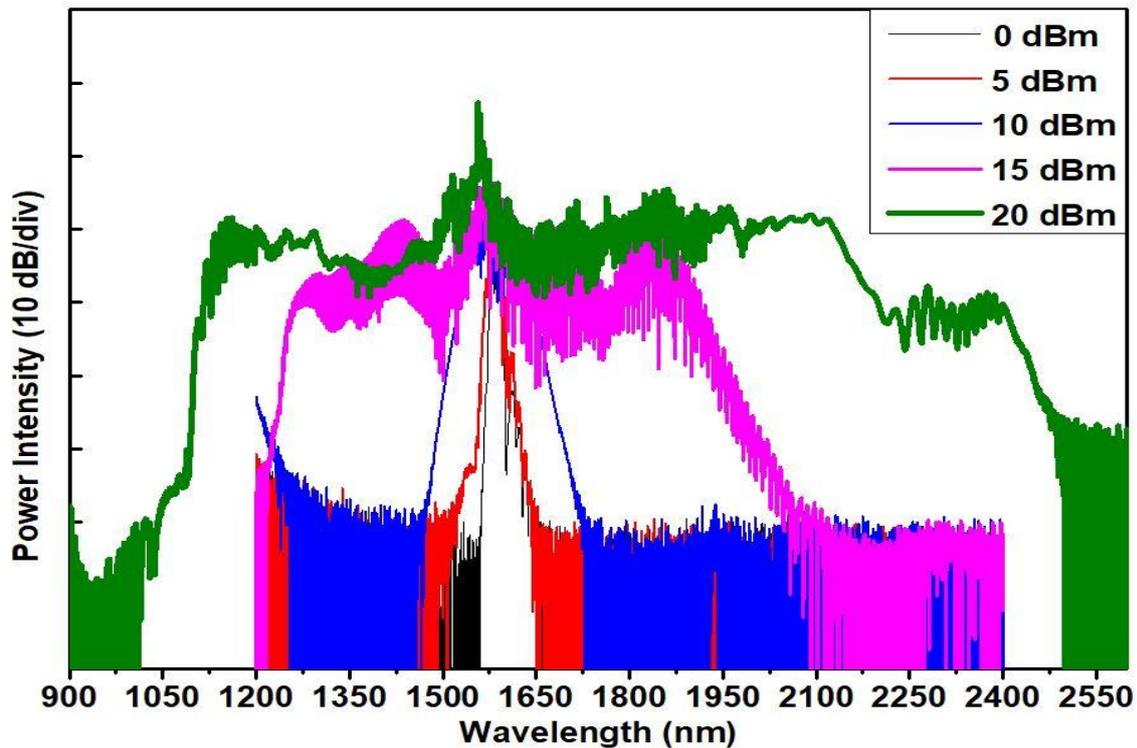
Figure 4. 9 Output SC spectral variation from 50-cm-long DS-HNLf for different input powers.
