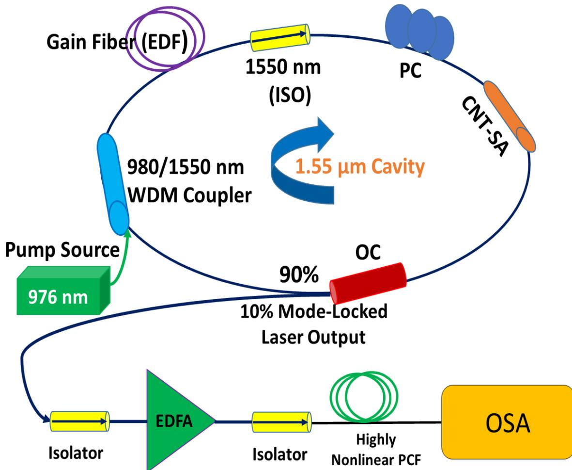
Figure 4. 2 Experimental setup of SC generation from a PCF using passively mode-locked fibre laser.
