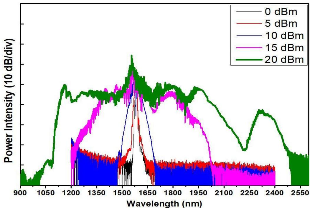
Figure 4. 15 SC spectral output from ~35-cm-long fibre ( $L_1 = 1$  cm and  $L_2 = 4$  cm).
