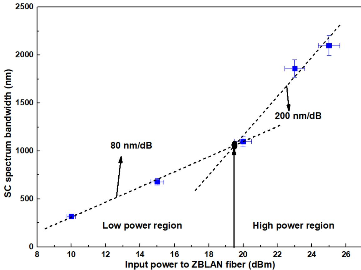
Figure 5. 4 SC spectrum bandwidth variation from 25-m-long ZBLAN fibre with respect to input pulse power variation.
