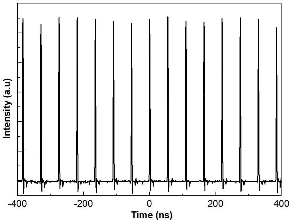
Figure 3 8 Optical pulse train of the mode-locked laser.
