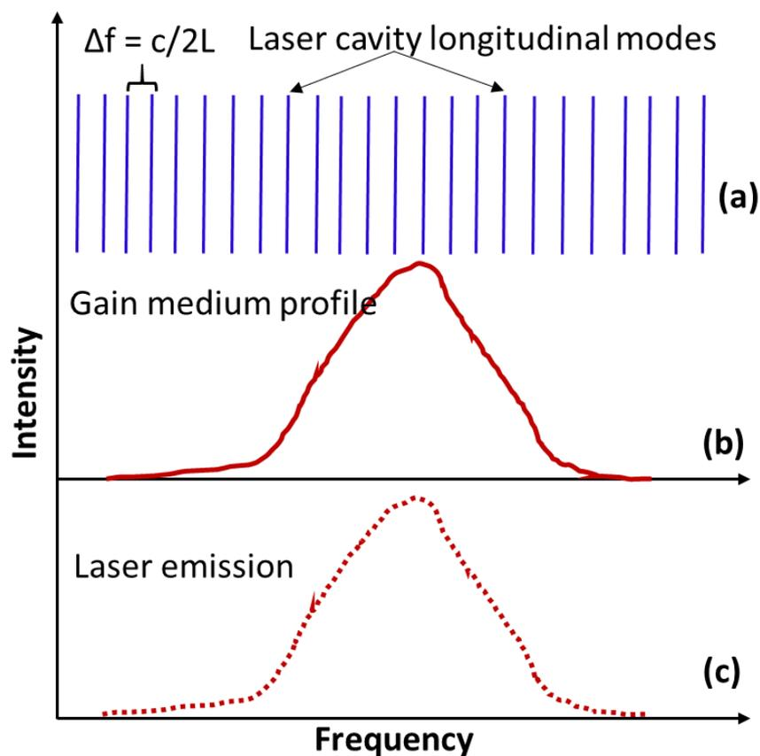
Figure 2. 2 The laser emission process: (a) Laser cavity longitudinal modes, (b) Laser Gain medium profiles, (c) laser emission frequency range
