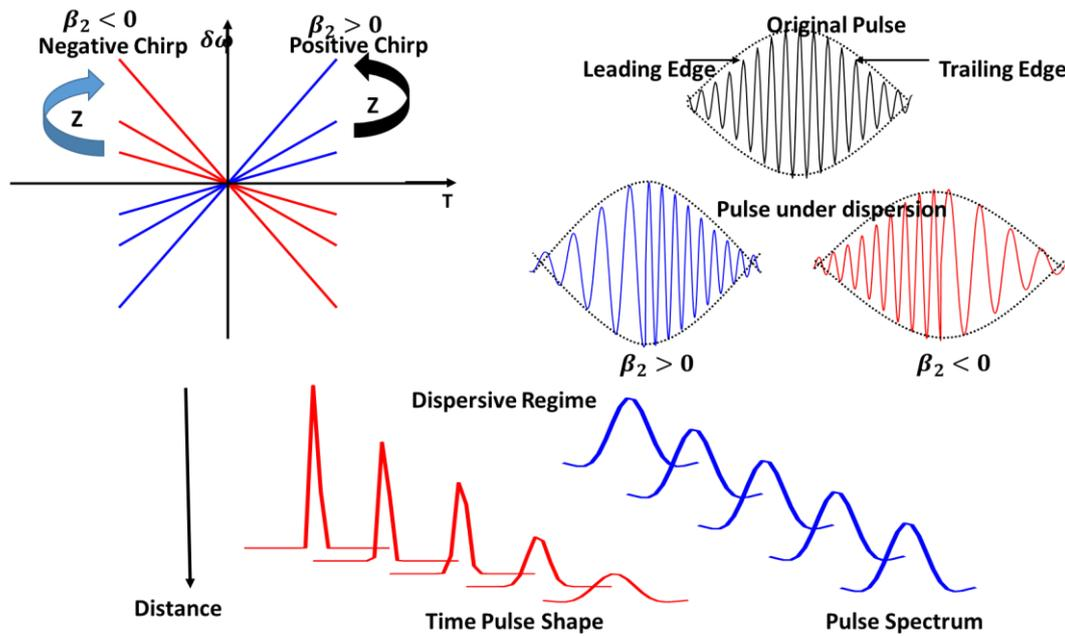
Figure 2. 13 Schematic illustration of pulse propagation through fibre in dispersive regime [59].
