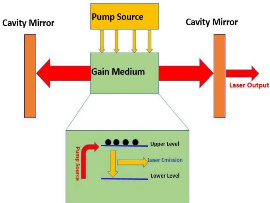
Figure 2. 1 Basic schematic of laser setup
