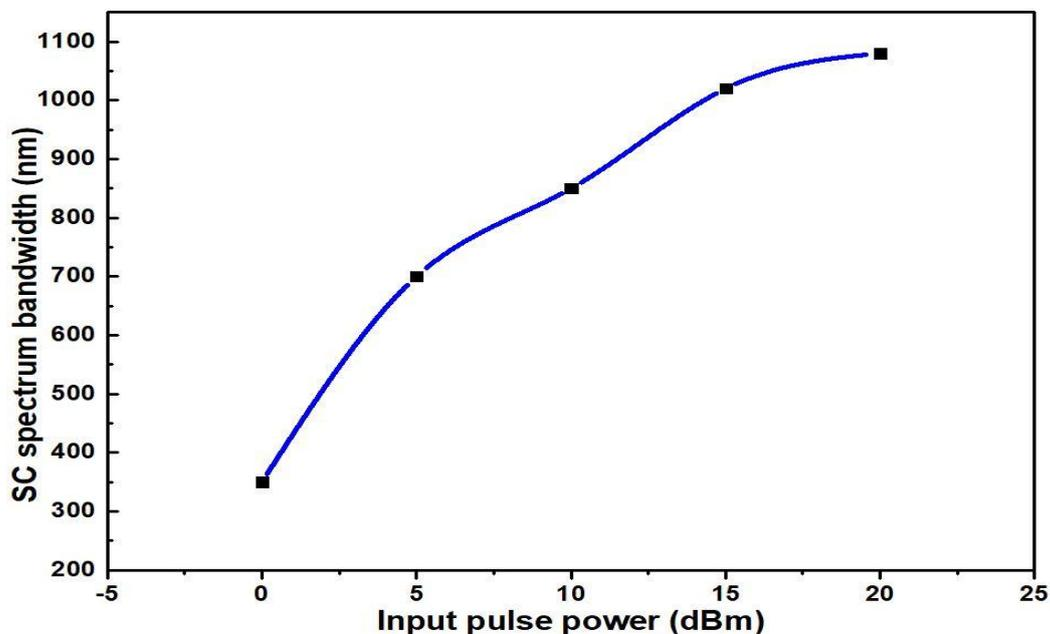
Figure 4. 4 PCF output SC bandwidth variation with respect to the input pulse power.
