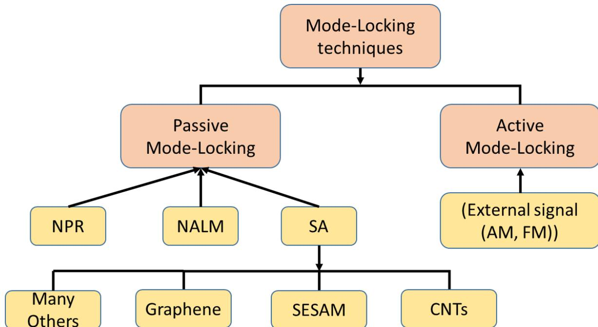
Figure 2. 6 Classification of mode-locking techniques: NPR: nonlinear polarization rotation, NALM: nonlinear amplifying loop mirror, SA: saturable absorber, SESAM: semiconductor saturable absorber mirror, CNTs: carbon-nanotubes, AM: amplitude modulator, FM: frequency modulator
