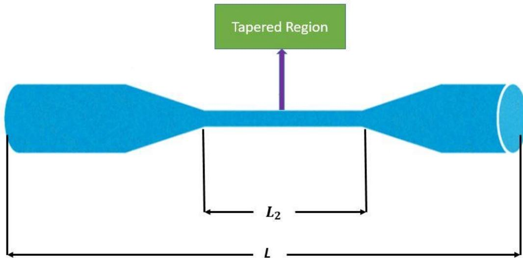
Figure 4. 14 Illustration of tapered fibre [133].
