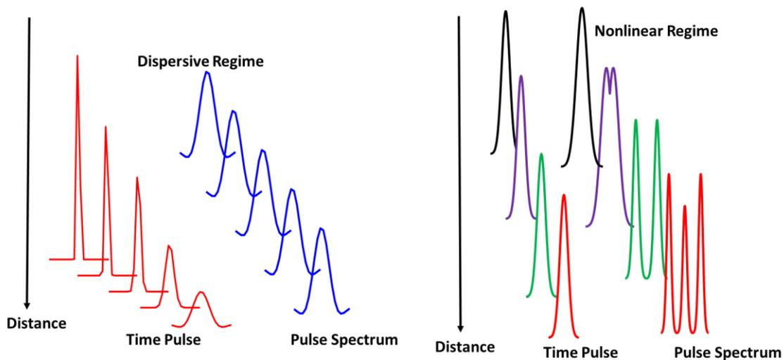
Figure 2. 15 Schematic illustration of pulse evolution in dispersive and nonlinearity regime [59].
