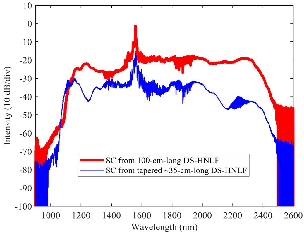
Figure 4. 17 SC spectrum from ~35-cm (6-cm-tapered) and 100-cm at the input pulse power of 20 dBm
