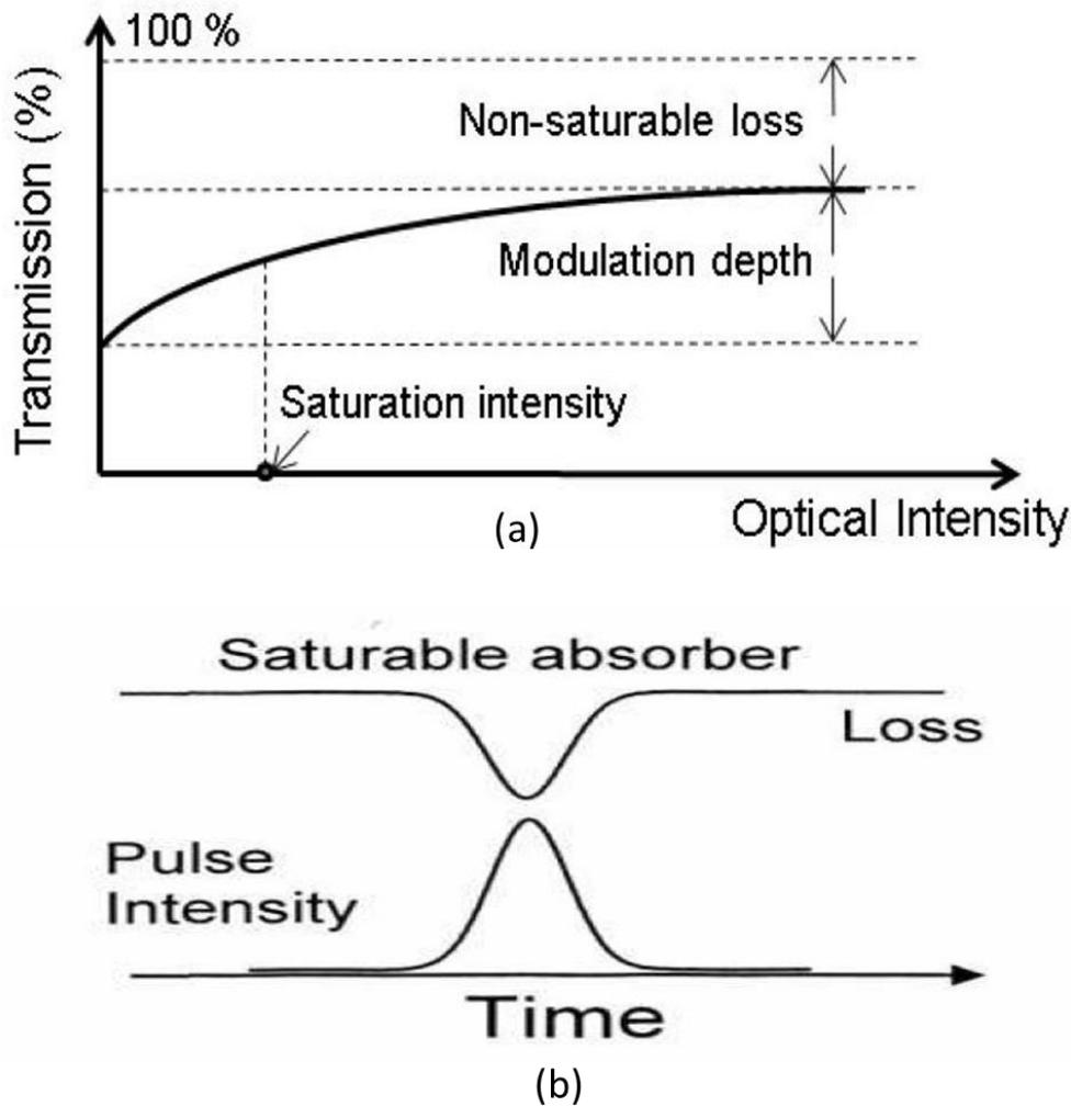
Figure 2. 9 Schematic representation of (a) SA nonlinear transmission (b) the SA-based pulse reshaping [51, 52].
