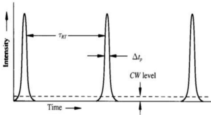
Figure 2. 4 Schematic of mode-locked laser emission.
