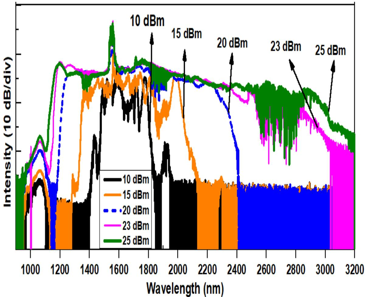
Figure 5. 3 SC spectrum output variation from 25-m-long ZBLAN fibre for different input pulse powers.
