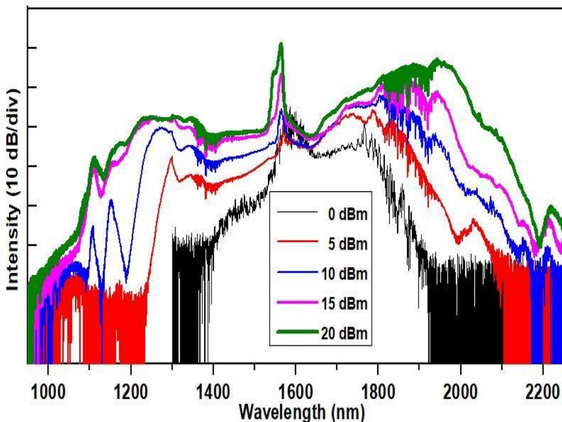
Figure 4. 3 SC spectrum output from PCF at different input pulse powers.
