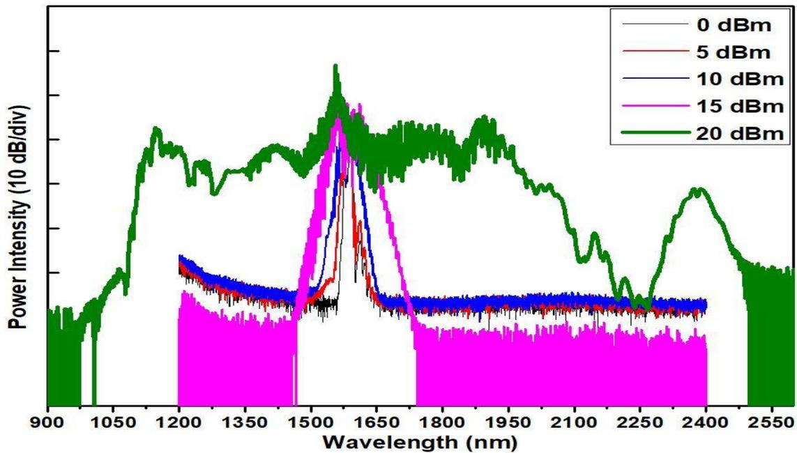
Figure 4. 8 Output SC spectral variation from 30-cm-long DS-HNLF for different input powers.
