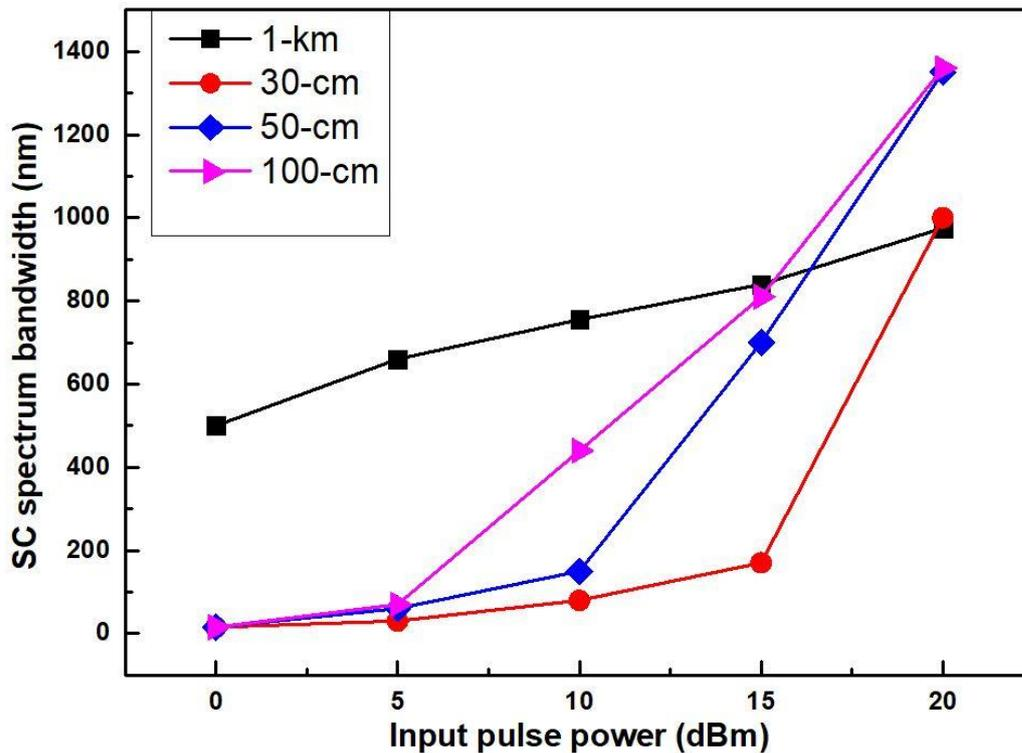
Figure 4. 11 SC spectral bandwidth variation from 30-cm, 50-cm, 100-cm and 1-km-long DS-HNLF with respect to the input power variation.
