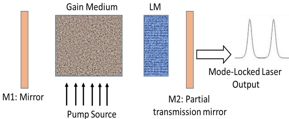
Figure 2. 5 Schematic of mode-locked laser: LM: Loss modulator.
