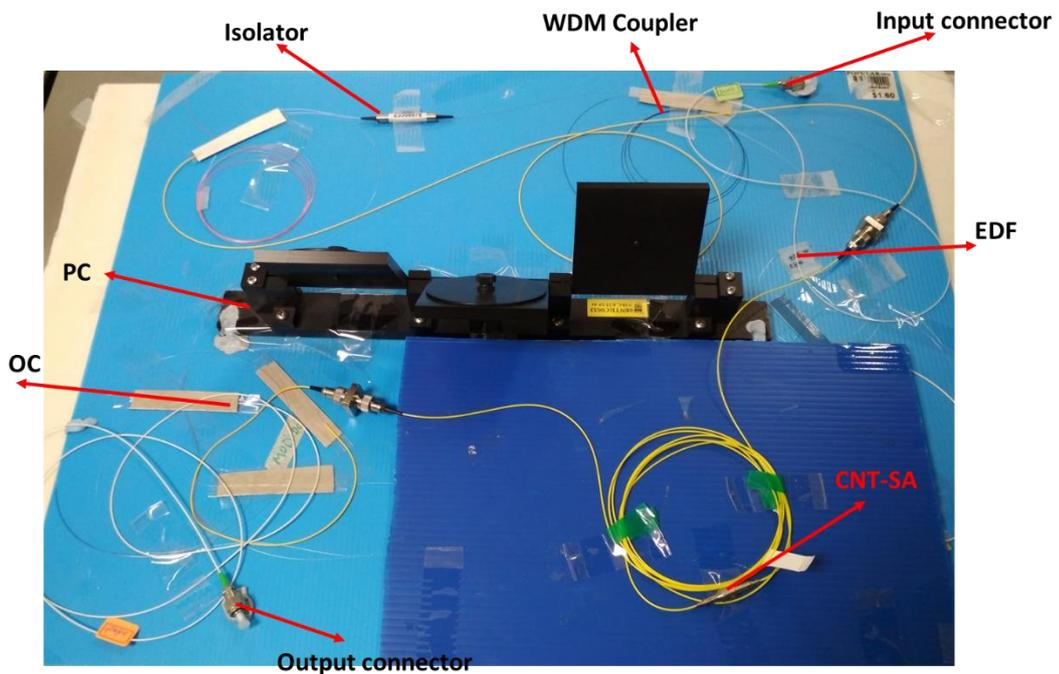
Figure 3. 5 Ring-cavity setup in the laboratory.
