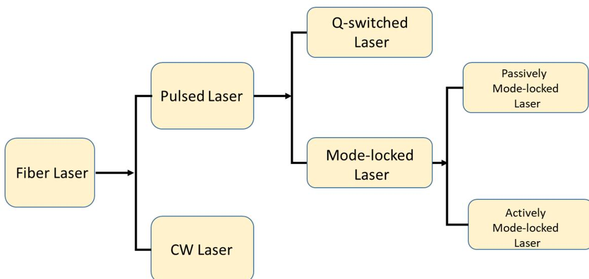
Figure 2. 3 Fibre laser classifications: CW: continuous wave.
