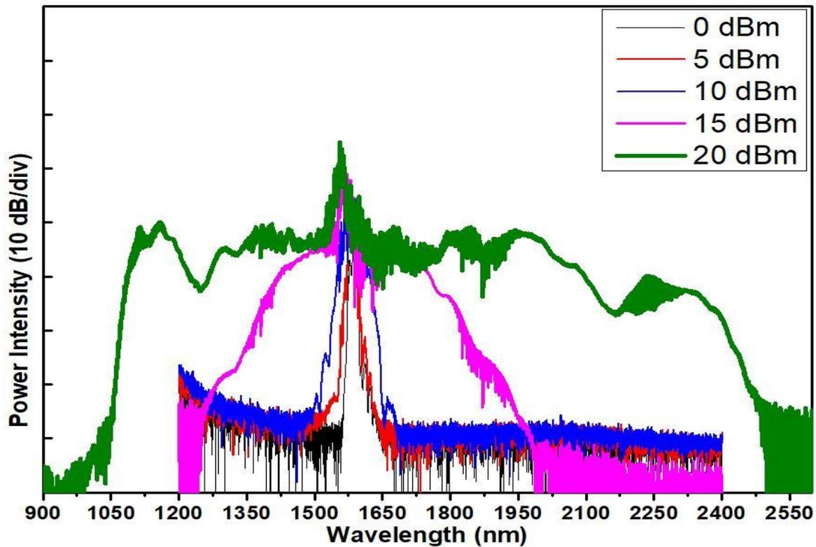
Figure 4. 16 SC spectral output from  $\sim 35$ -cm-long fibre ( $L_1 = 1.5$  cm and  $L_2 = 6$  cm).
