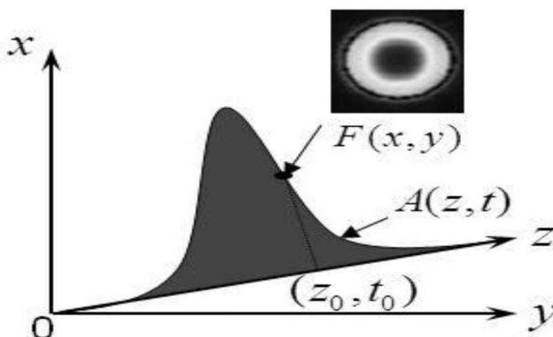
Figure 2. 12 Graphical representation of an optical pulse electric field. [51]
