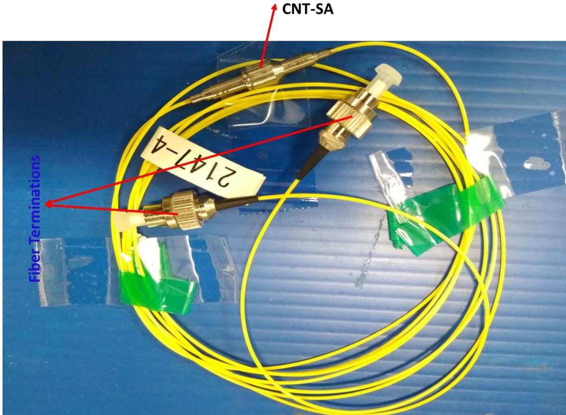
Figure 3. 4 CNT-SA used for the passive mode-locking.
