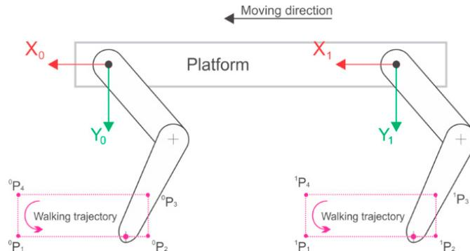
Fig. 5. Rectangular shape trajectory was chosen as walking trajectory for its simplicity.
