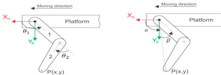
Fig. 4. Frame allocation of the simplified model of the leg with notations for different joint angles
