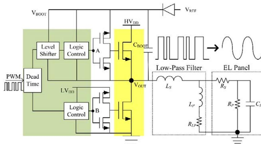
Fig. 1. Class-D driver for EL panel
