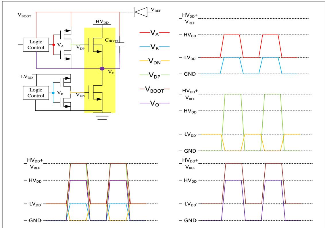
Fig.2. The signal waveforms of the Class-D driver
