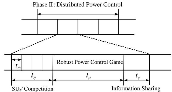
Fig. 3: Implementation in a time slotted frame structure.
