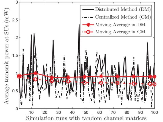
Fig. 9: Average transmit power is higher in the distributed method.
