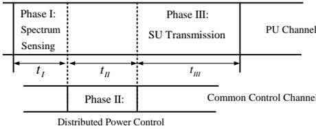
Fig. 2: SUs' channel access in time slotted structure.
