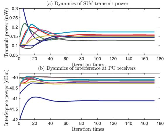
**Fig. 5:** Dynamics of Algorithm 1 with  $N = 8$  SUs and  $K = 8$  PUs.
