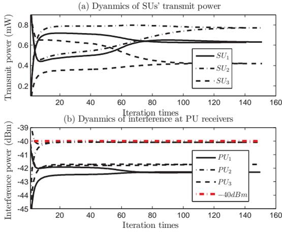
**Fig. 4:** Dynamics of Algorithm 1 with  $N = 3$  SUs and  $K = 3$  PUs.
