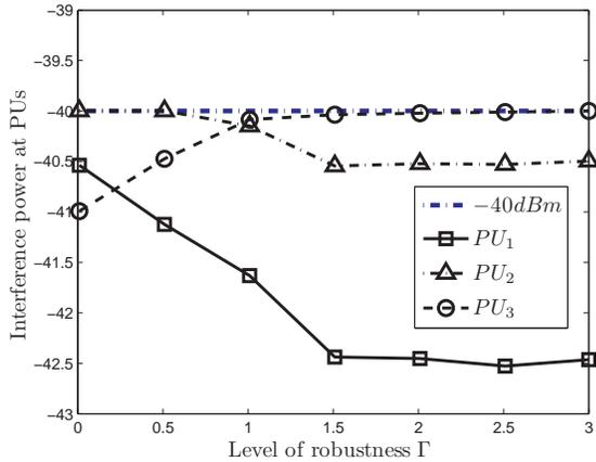
Fig. 11: Interference power at PU receivers.
