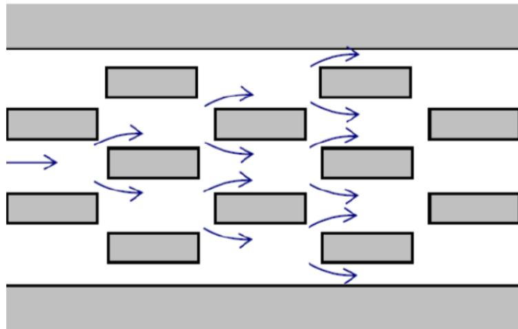
Figure 1: Fluid flow about an offset fin geometry [1]
