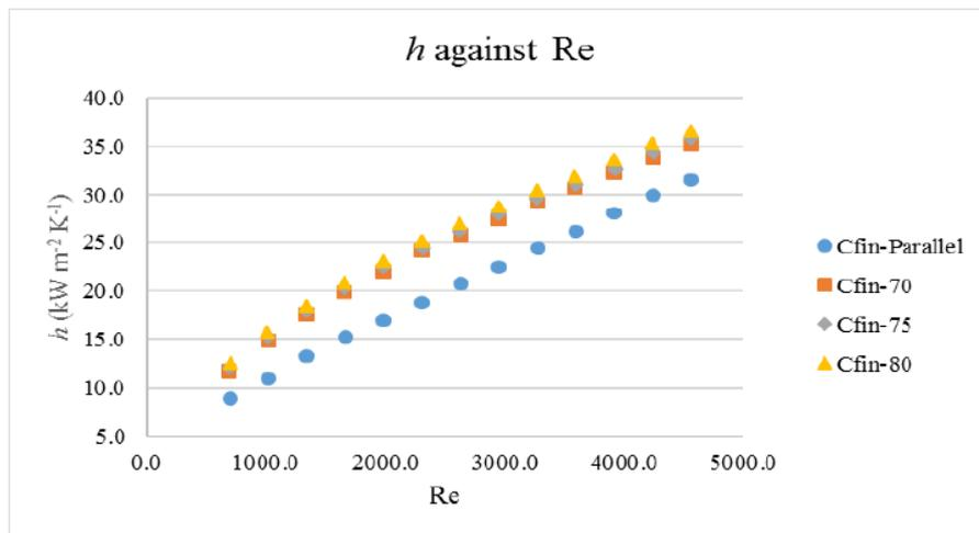
Figure 8: Heat transfer coefficient against Reynolds number
