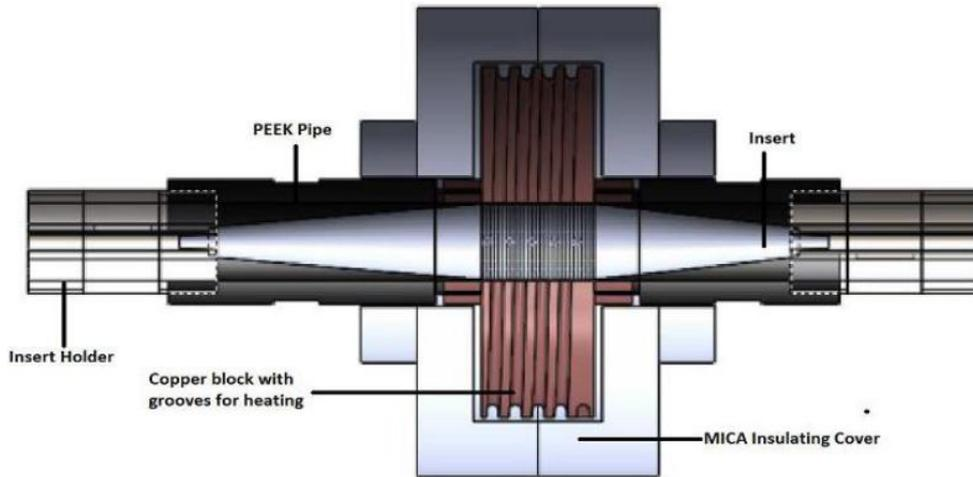
Figure 3: Key components of the test module
