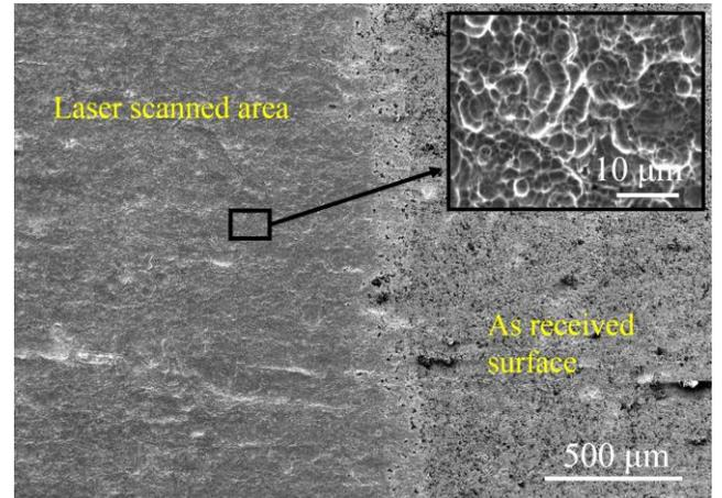
Fig. 2. SEM image showing the AMS 4911 surface before and after laser cleaning (the inset shows blow up image of the laser cleaned surface). Laser fluence of  $0.068 \text{ J/cm}^2$  at the surface was used for cleaning.
