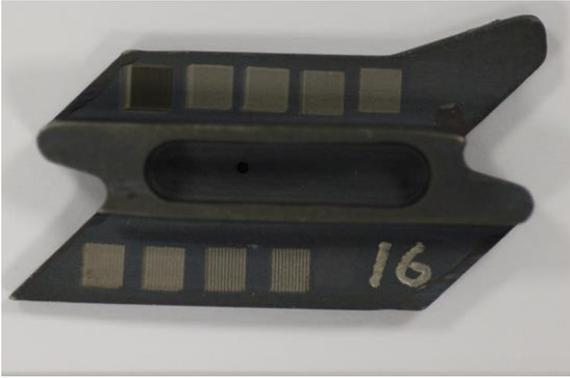
Fig. 1. Femtosecond laser cleaning at different laser conditions in air (top: titanium alloy; bottom: nickel superalloy based turbine blade).
