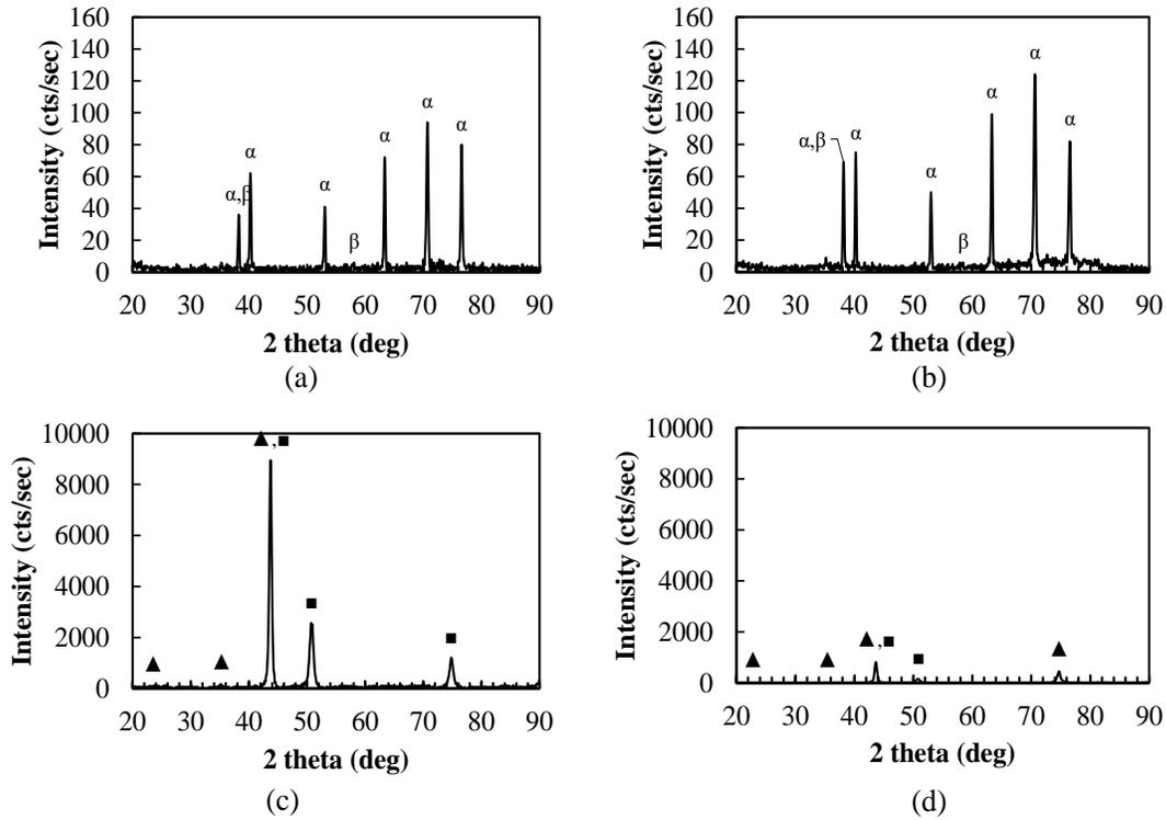
Fig. 4. XRD results. (a) and (b) are the X-ray diffractograms of AMS 4911 alloy before and after laser cleaning respectively.  $\alpha$  represents alpha-phase and  $\beta$  represents beta-phase in the alloy. Similarly, (c) and (d) are the X-ray diffractograms of turbine blade before and after laser cleaning respectively.  $\blacktriangle$  represents AlNi<sub>3</sub> phase while  $\blacksquare$  represents Al<sub>0.5</sub>CNi<sub>3</sub>Ti<sub>0.5</sub> phase.
