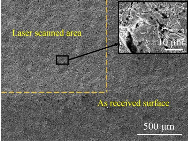
Fig. 3. SEM image showing the turbine blade surface before and after laser cleaning (the inset shows blow up image of the laser cleaned surface). Laser fluence of 0.367 J/cm<sup>2</sup> was used.
