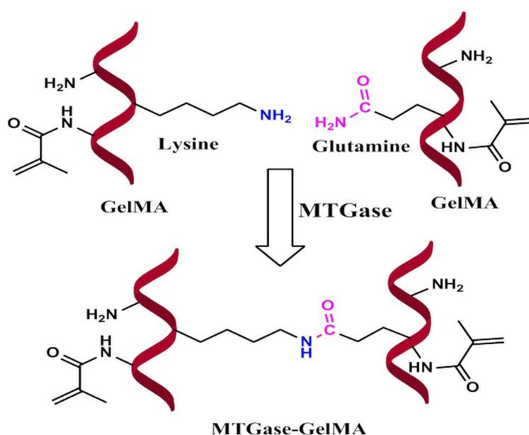
**Figure 2.** The crosslinking mechanism of the MTGase-GelMA hydrogel
