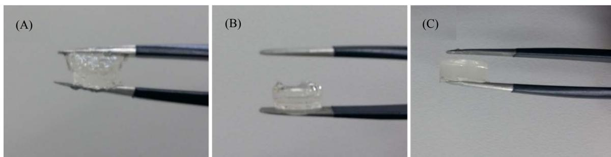
**Figure 6.** Handling of (A) enzymatic, (B) photo- and (C) dual crosslinked hydrogels
