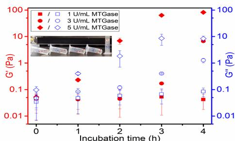
**Figure 3.** Effect of the MTGase concentration on the gelling period of 10% GelMA solutions at incubation temperature (37 °C). The inset photo shows representative images of transition from a liquid to a chemical gel of 10% GelMA treated with 3 U/mL MTGase at 37 °C.
