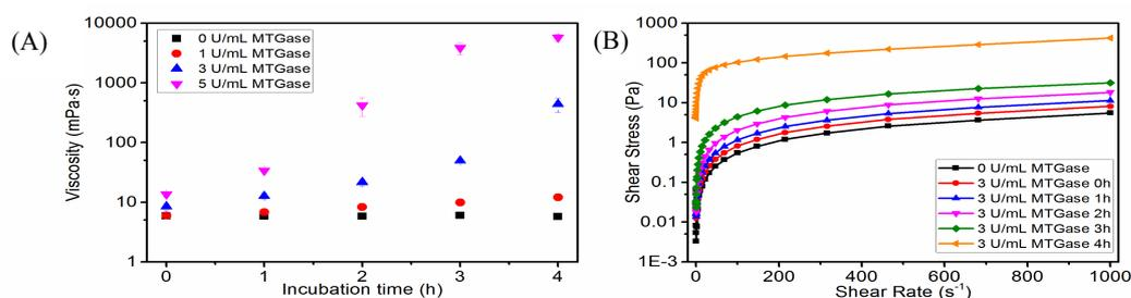
**Figure 4.** (A) The time-dependent viscosity of 10% GelMA solution incubated with different concentration of MTGase at 37 °C under the shear rate of  $100 \text{ s}^{-1}$ ; (B) the flow behaviour of 10% GelMA solution incubated with 3 U/mL MTGase at 37 °C
