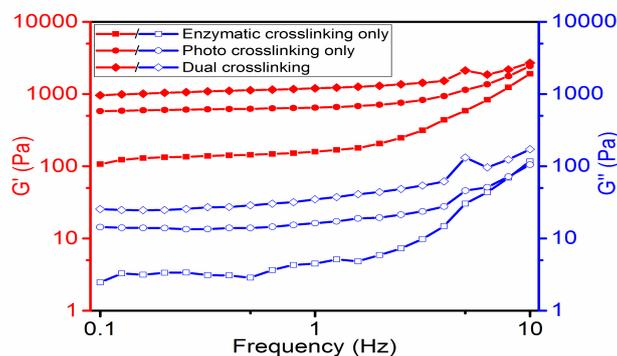
**Figure 5.** Viscoelastic properties of different crosslinked hydrogels. Enzymatic crosslinking hydrogel was formed by incubating 10% GelMA with 3 U/mL MTGase for 12 h. Photo crosslinking hydrogel was formed by curing 10% GelMA at 1.5 mW/cm<sup>2</sup> for 5 min. Dual crosslinking hydrogel was formed by enzymatic crosslinking and then by photo crosslinking.
