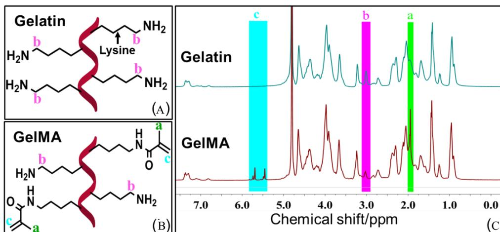
**Figure 1.** The chemical structures of (A) unmodified gelatin and (B) GelMA, and (C) their respective  $^1\text{H-NMR}$  spectra. Green “a” and blue “c” represent the signals of the methyl group and acrylic protons of the grafted methacrylic group respectively, and pink “b” indicates the signal of lysine methylene.
