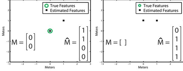
Fig. 1. Hypothetical scenario showing a fundamental inconsistency with vector representations of feature maps. If  $M$  is the true map, how should the error be assigned when the number of features in the map estimate,  $\hat{M}$ , is incorrect?
