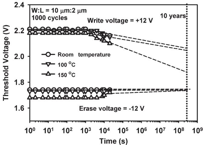
Fig. 4. Data retention characteristics at various temperatures. The devices have been programmed/erased for 1000 cycles at +12 V/−12 V with a pulse width of 1 ms.
