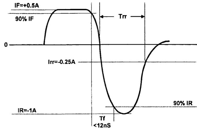
Fig. 3. Current waveform in RG1 reverse recovery test circuit.
